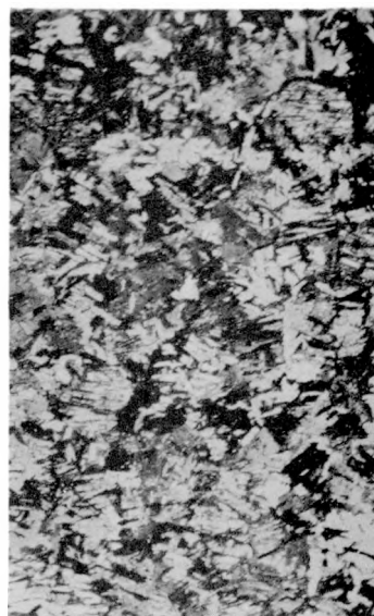
Fig. 14(b) - Sample cold-drawn 15% and oxidized 10 seconds by resistance heating. No gross oxide layer formed.
