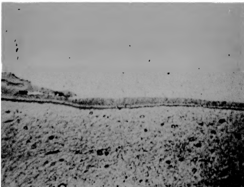
Fig. 1 - Interface in copper clad Zircaloy tube, as-extruded, showing alloying in diffusion zone; two sections, copper at top.
