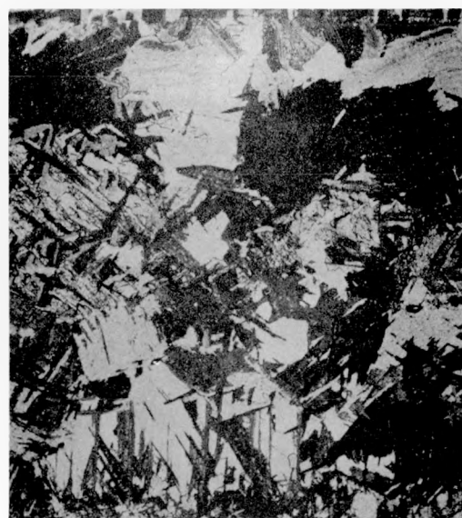
Fig. 14(a) - As-extruded sample oxidized by resistance heating for 20 seconds. Marked oxide layer is observable.
