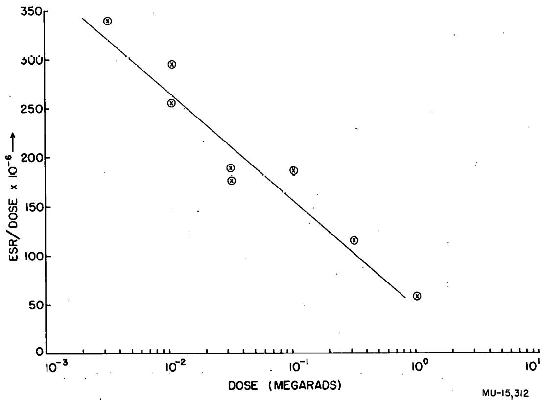
Fig. 16. ESR signal yield vs dose for irradiated choline chloride.
