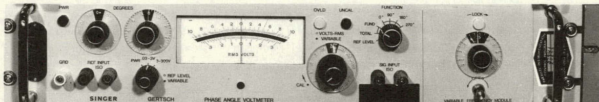
Figure 3. PHASE-ANGLE VOLTMETER USED IN THE TRANSFER-RATIO MEASURING CIRCUIT.
