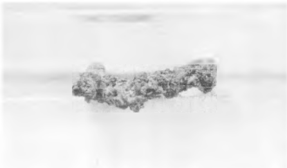
Fig. 5—An irradiated uranium-10 wt. % plutonium alloy specimen cooled slowly through the beta-alpha transformation. This specimen is similar to specimen BG-5, which ignited before being photographed. (Magnification 2 \times .)
