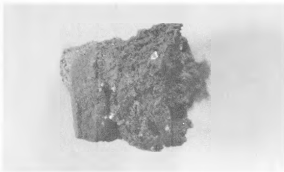
Fig. 4—Specimen G-20, a hot-pressed unalloyed uranium compact, with a total atom burn-up of 0.53 per cent (4500 Mwd/ton). The specimen ignited about 35 min after this photograph was taken. (Magnification 2 \times .)
