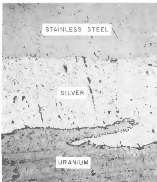
Fig. 28—Stainless steel-silver-uranium interface. (Magnification 500×.)
