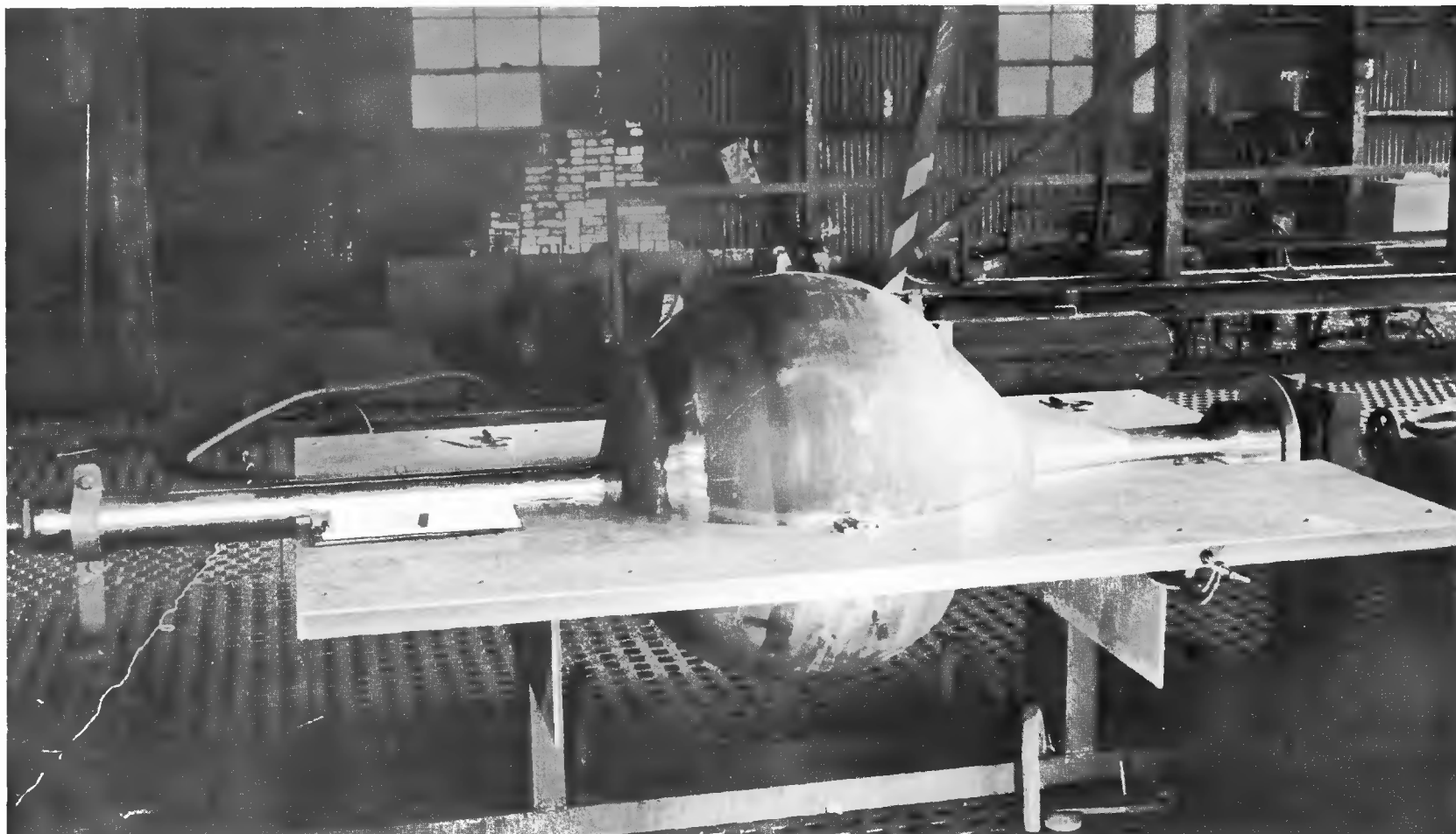
Fig. 28— Making dimensional check of outside of vessel. Measurements of both radius and thickness were made and recorded every 15 deg. Thickness measurements were made by a calibrated audigauge. Radius readings were taken before and after the hydrostatic test.
