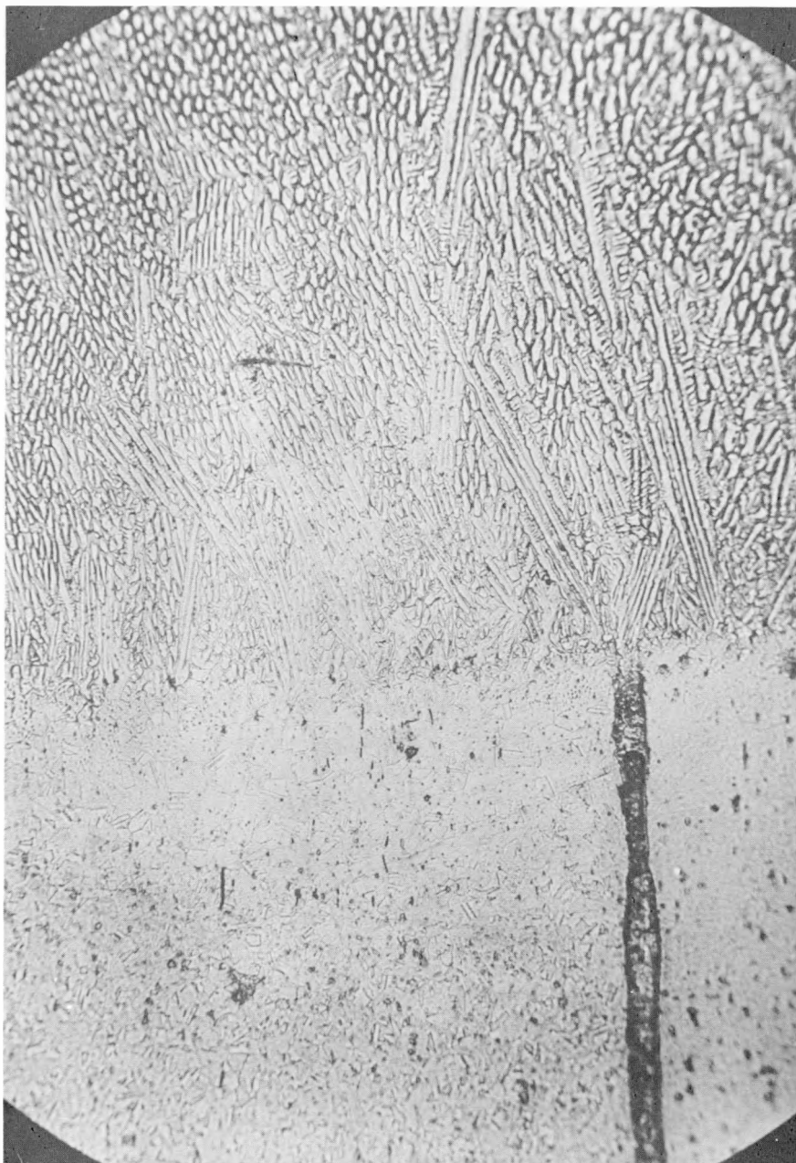
Fig. 29—Cross section of weld. (Magnification 500 \times .)
