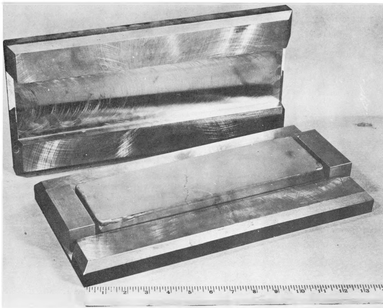
Fig. 20—Welded cladding billet in steel sheath. The welded billet is sealed in a steel sheath to prevent surface contamination of the billet while rolling.
