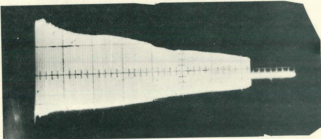
Fig. 3. Sweep trigger--end of rectification. Sweep speed 200 msec/cm. Sum induction-electrode signal of circulating proton beam tracked during the inversion period from 6.2 Bev down to 300 Mev.
