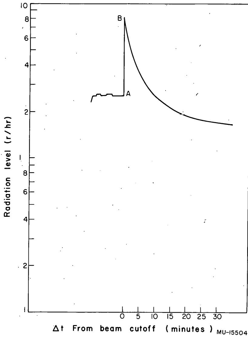
Fig. 4. Typical radiation decay on Speedomax chart.
