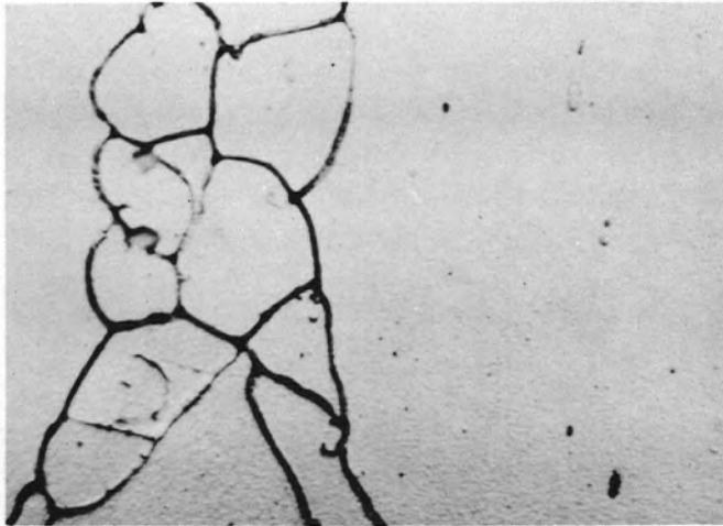
(a) Inconel X heated to 2400°F and fractured at 2000°F 1000X
