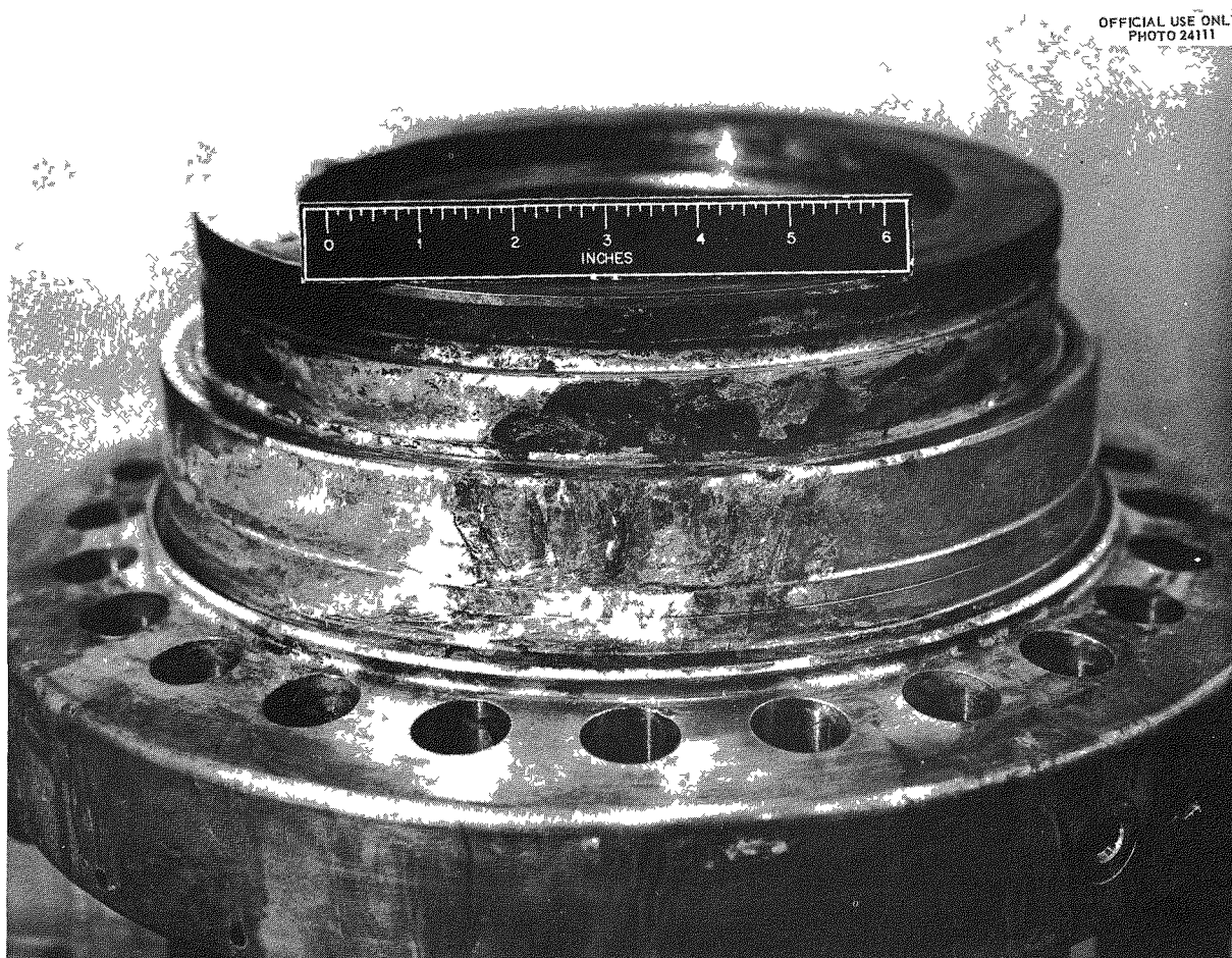
Fig. 4.6. HRT Mockup Pump Stator Assembly.
