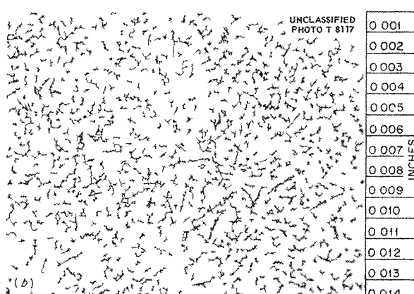
Fig. 13.6. (a) As-Welded Type 347 Stainless Steel Containing 5 to 6% Ferrite. (b) Original 5 to 6% Ferrite Heat Treated at 1250°F, 48 hr; Less Than 1% Ferrite Remaining.
