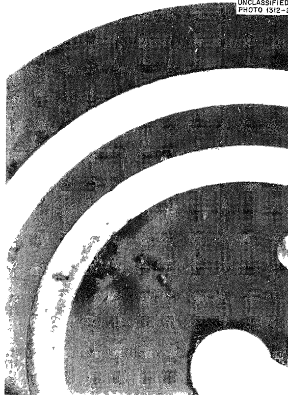
Fig. 10.2. Enlarged View of Section of Gold-Plated Iso-Elastic Spring Showing Blister Formation After Exposure in Boiling 0.17 m UO_2SO_4 Solution. 5X. Reduced 32%.
