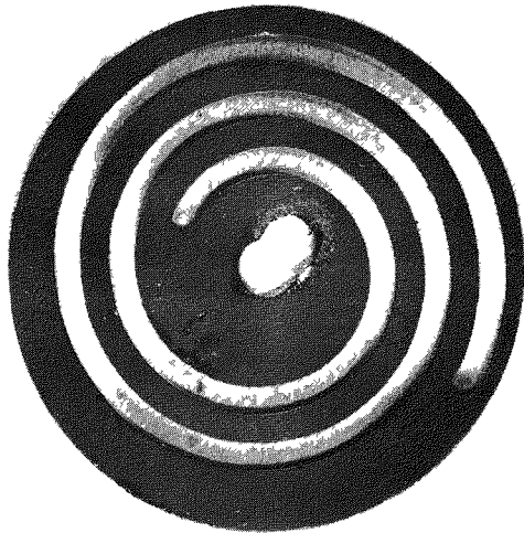
Fig. 10.1. View of Gold-Plated Iso-Elastic Spring Showing Corrosion Damage After 120 hr in Boiling 0.17 m UO_2SO_4 Solution. 2X. Reduced 29%.
