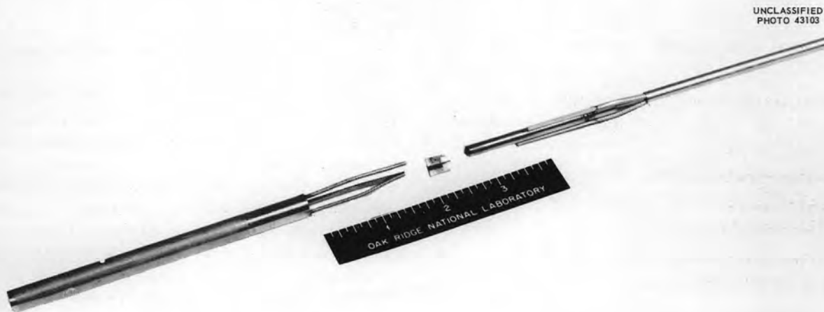
Fig. 163. INOR-8 Capsule for Corrosion Studies in the MTR.
