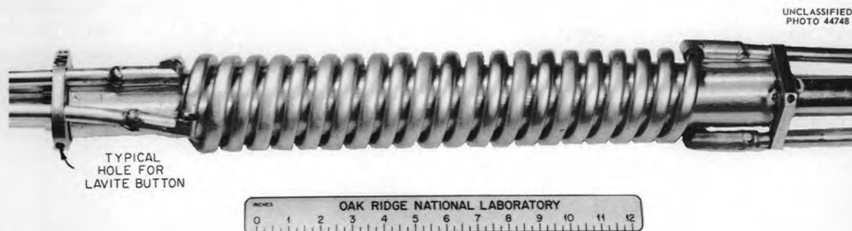
Fig. 76. Expansion Coil for Hole 50 Cryostat.
