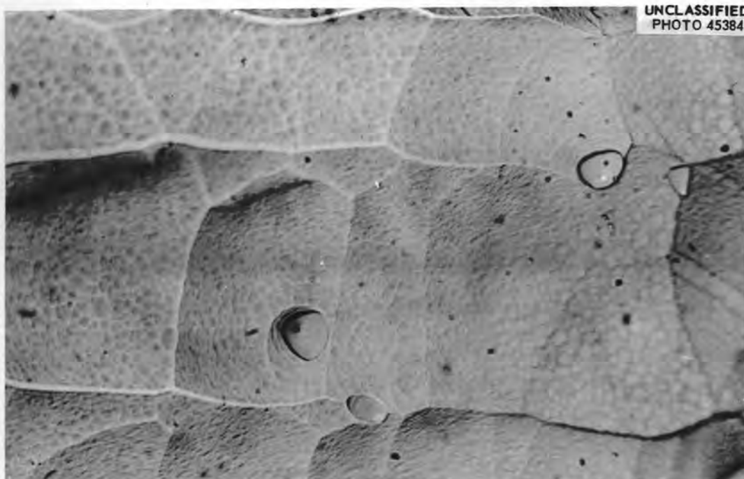
Fig. 12. Unirradiated p -Type Germanium, (111) Face. Bromine-enriched CP-4 etch. 500X.
