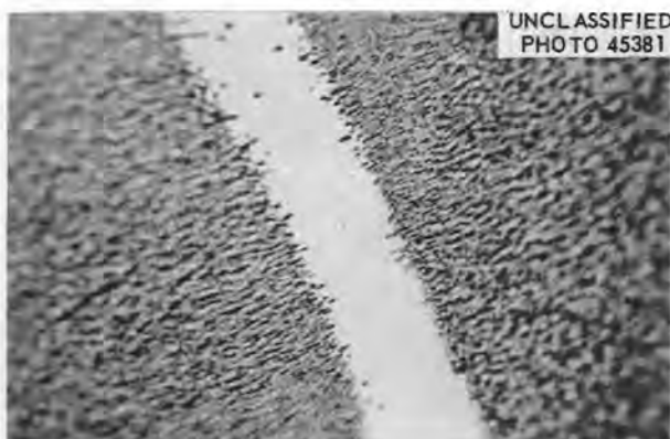
Fig. 82. (110) Pole of Copper Hemisphere Etched in 0.5 M KCN for 45 min. 500X.
