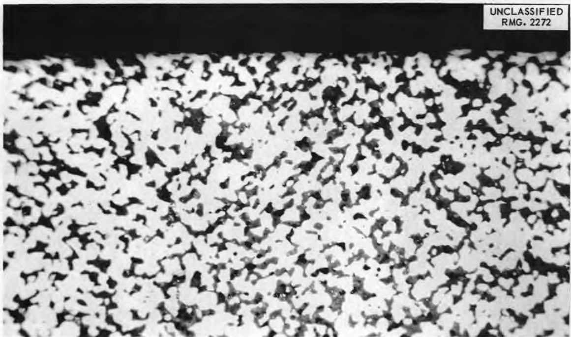
Fig. 137. Exterior Surface of UO 2 Fuel Plate Clad with Cr-Al 2 O 3 . 500X.
