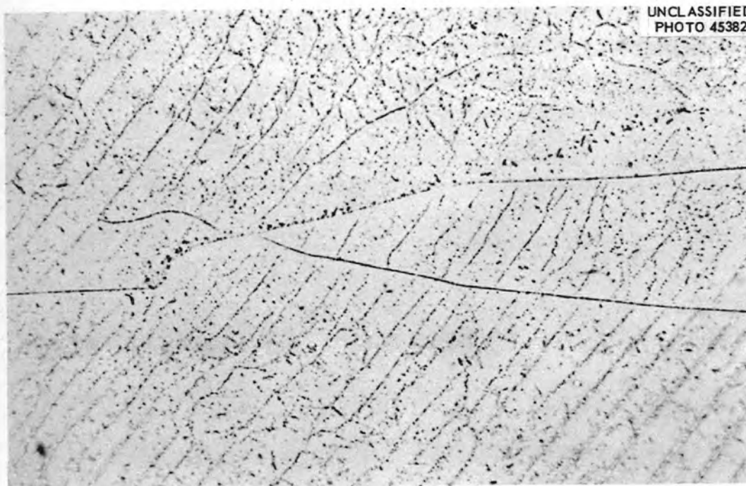
Fig. 81. Electrolytic Etch Pits on Same Area as Fig. 80. 500X.
