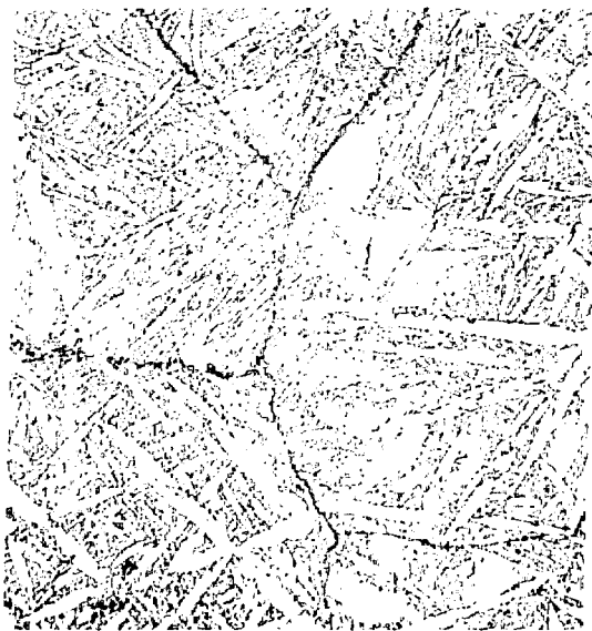
Fig. 13. Microstructure (250X) of quenched and aged U-0.83 wt% Ti alloy tensile-test specimens. Left, oil-quenched; right, water-quenched.
