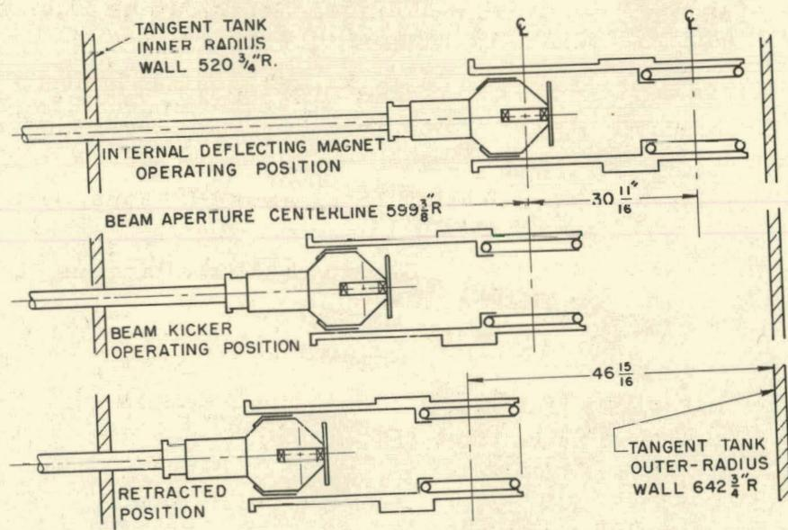
Fig. 11. Schematic diagram showing how the internal deflecting magnet and the rapid beam-ejector magnet share the same positioning apparatus.
