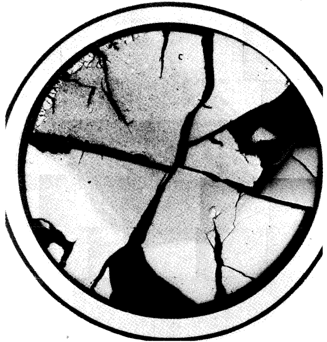
Fig. 463-1. Photomosaic of a high-density, sodium-bonded, carbide fuel element showing asymmetric regions of grain-boundary swelling. (Fuel element U194, Section F; Mount No. 2C8).
