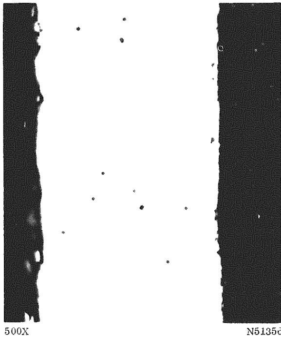
a. Iron-46.25 w/o Chromium Heated 720 Hr at 650 C and Water Quenched
