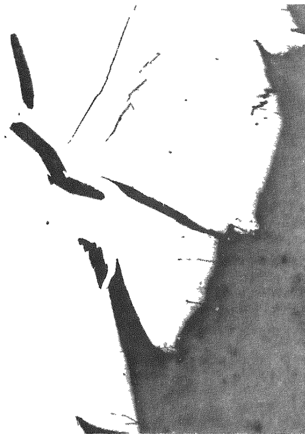
FIGURE 39. AUXILIARY CRACKS IN AN IRON-35 w/o CHROMIUM-6 w/o ALUMINUM ALLOY
