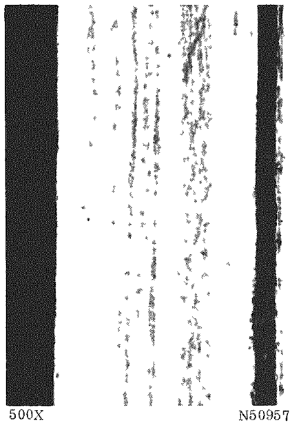
c. Iron-50 w/o Chromium Heated 1600 Hr at 500 C and Water Quenched
