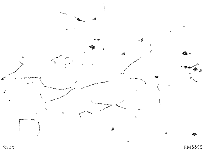
FIGURE 27 IRON-25 w/o CHROMIUM-5 w/o ALUMINUM ALLOY ANNEALED 1 HR AT 1000 C AND ROLLED 20 PER CENT AT 25 C
