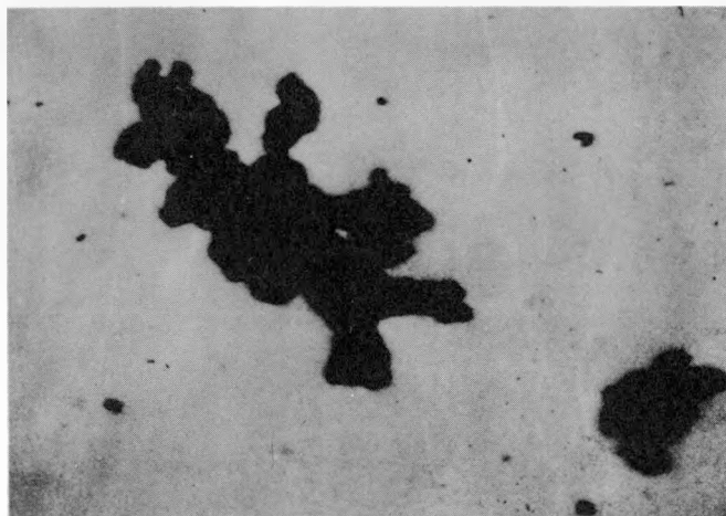
Fig. 1—Electron micrograph (10,000 \times ) of uranium powder produced by the hydride process. It can be seen that most of the particles are smaller than 1\ \mu and that there is a tendency for agglomeration.
