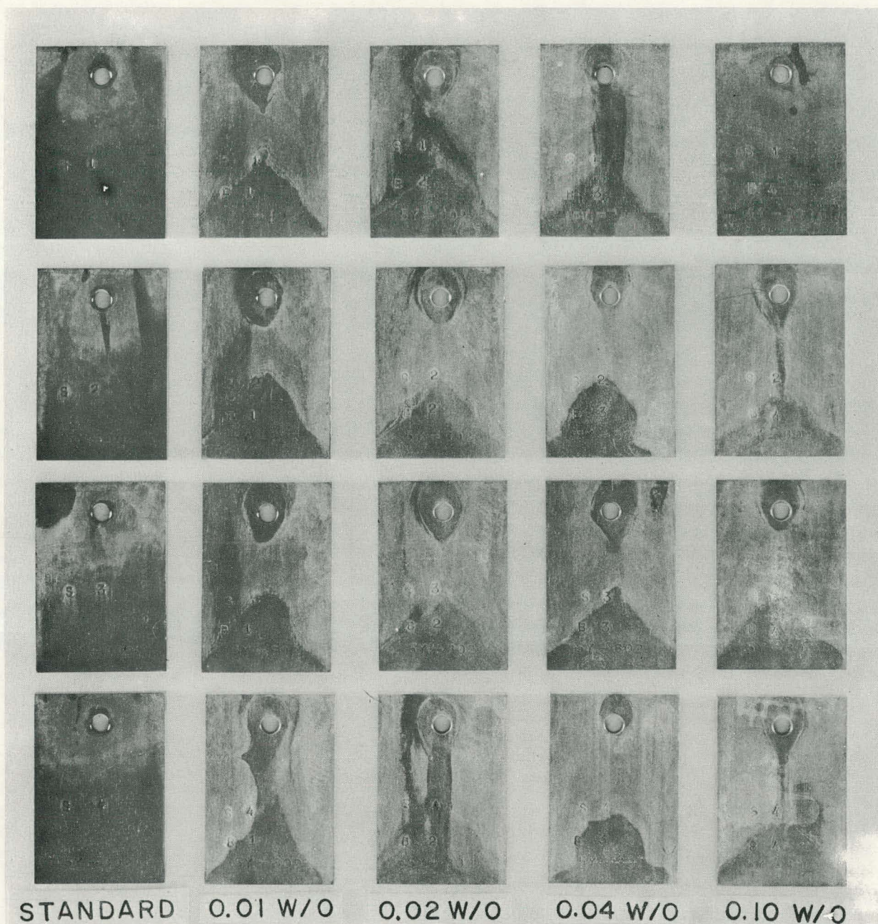
Fig. 16 Zircaloy-2 Corrosion Coupons Corrosion Tested for 10 Days in 750°F, 1500 psi Steam; Swift Akweons 674, Slow Rinse (Neg 23311-2)
