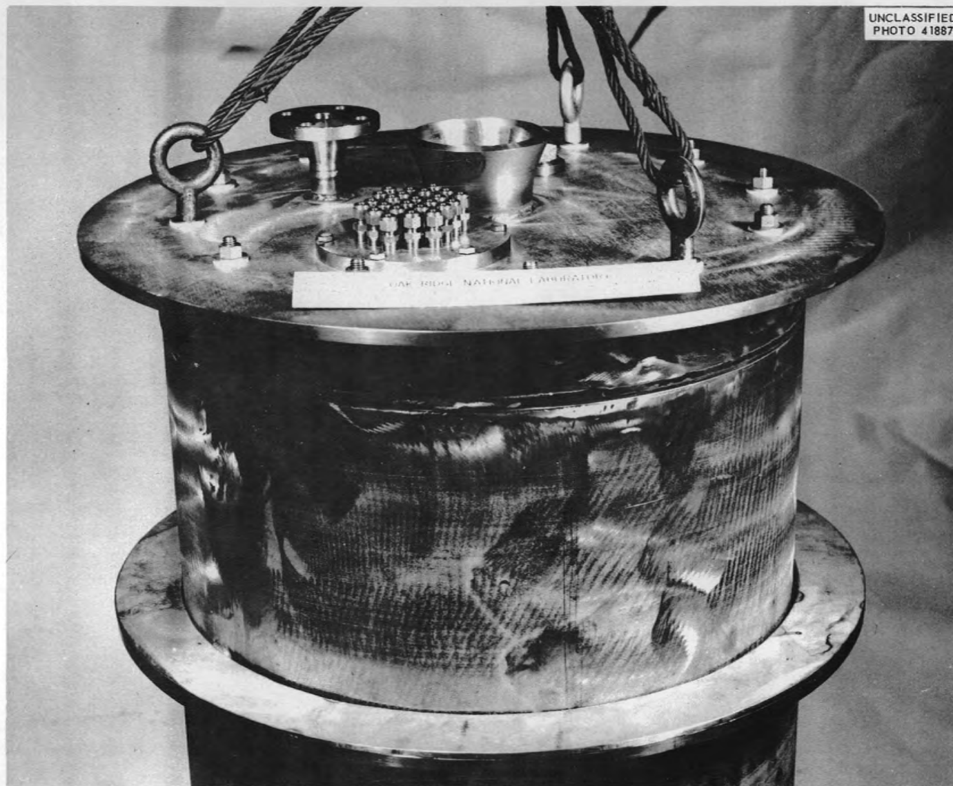
Fig. 30. "Adiabatic" Furnace, Showing Inner Container and Cover.
