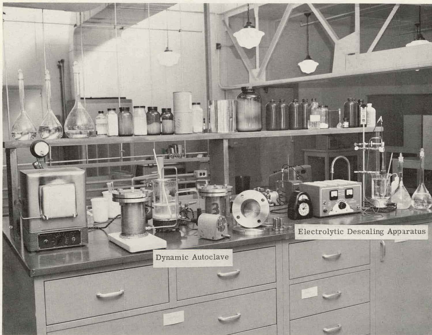
Fig. 1 Laboratory Bench Facilities For Dynamic Autoclave and Electrolytic Descaling Testing
