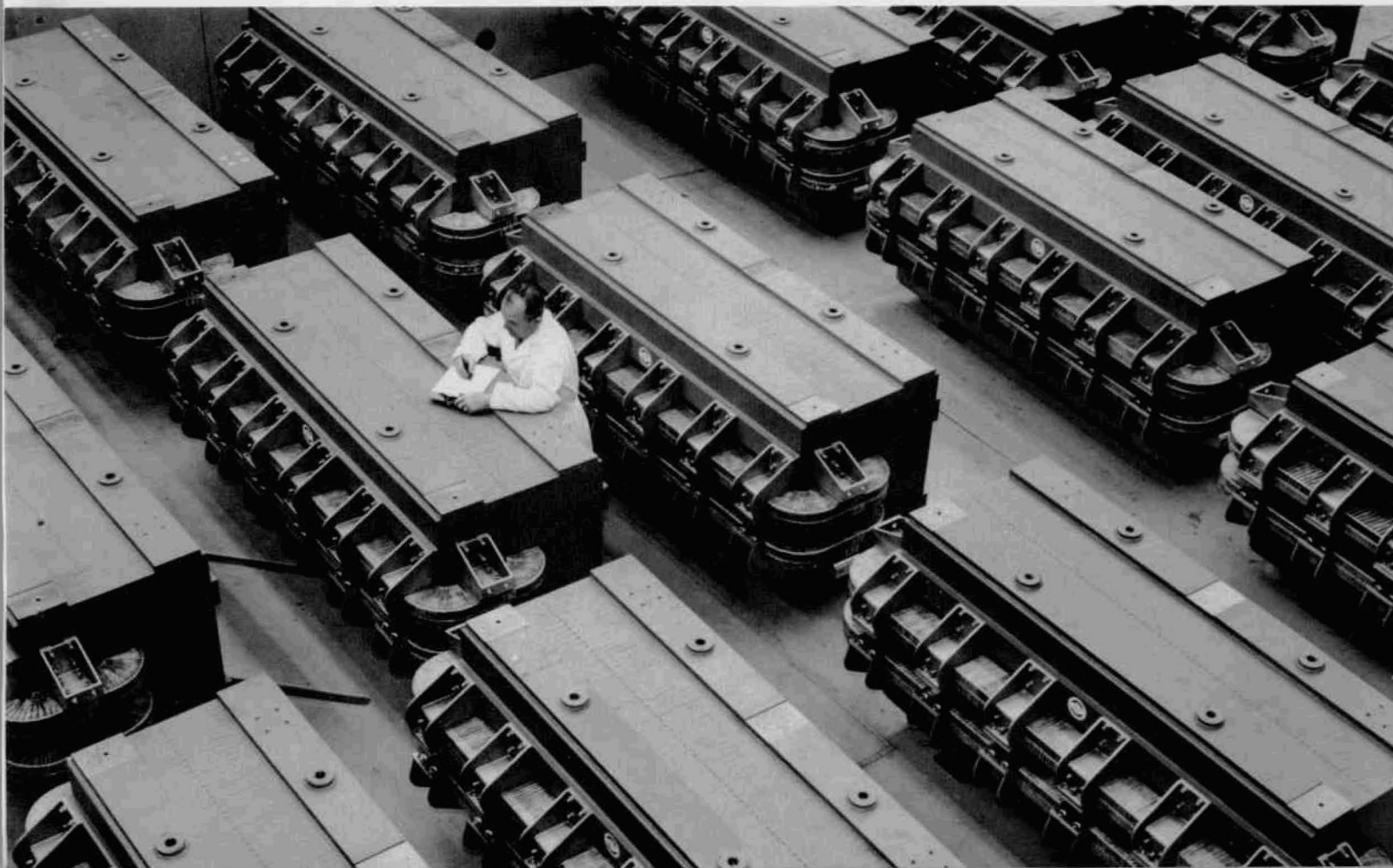
Figure 7. Some of the 240 magnets of the Alternating Gradient Synchrotron with coils attached prior to tests.
