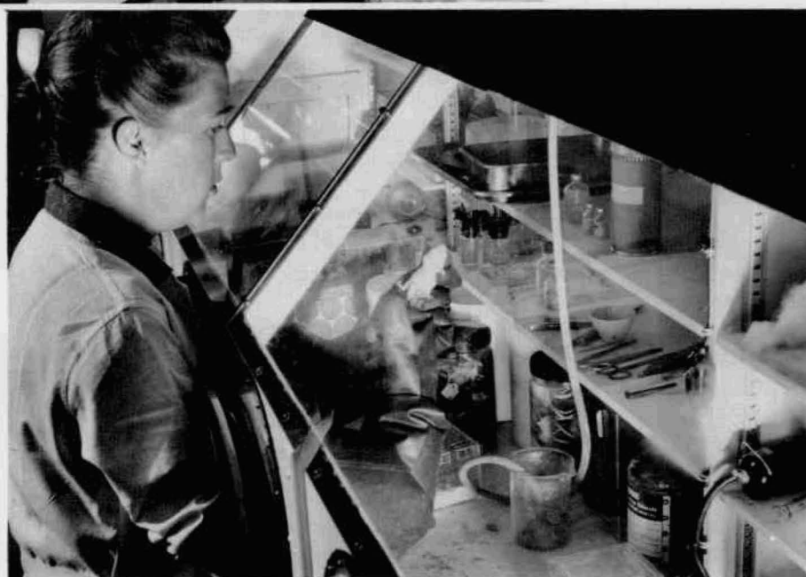
Figure 1. Small, self-contained laboratory and animal quarters for use in experiments with tritium-labeled thymidine and other radioactive materials. The labeled thymidine has proved of great value in the study of the synthesis of deoxyribose nucleic acid, a constituent of chromosomes, and in the study of chromosome formation during cell division. Although the radiation from the tritium is weak, a property that makes it uniquely suitable for localization of labeled material by autoradiography, the concentrations required are relatively high and potentially dangerous, particularly when the tritium is a component of material of long biological lifetime, such as thymidine. Experimental animals, equipment, and other materials are introduced at the left. During the course of an experiment, the operator works with gloved hands within the box. Contaminated and used material and material for further study are removed from the box through a door at the right. A slow stream of air is drawn through the box at all times.
