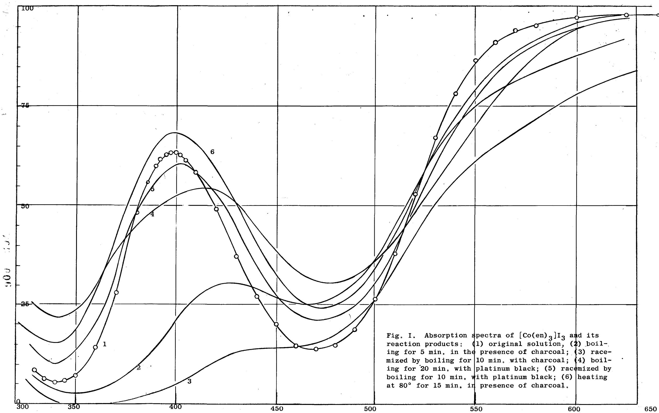
Fig. I. Absorption spectra of  $[\text{Co}(\text{en})_3]\text{I}_3$  and its reaction products: (1) original solution, (2) boiling for 5 min. in the presence of charcoal; (3) racemized by boiling for 10 min. with charcoal; (4) boiling for 20 min. with platinum black; (5) racemized by boiling for 10 min. with platinum black; (6) heating at  $80^\circ$  for 15 min. in presence of charcoal.
