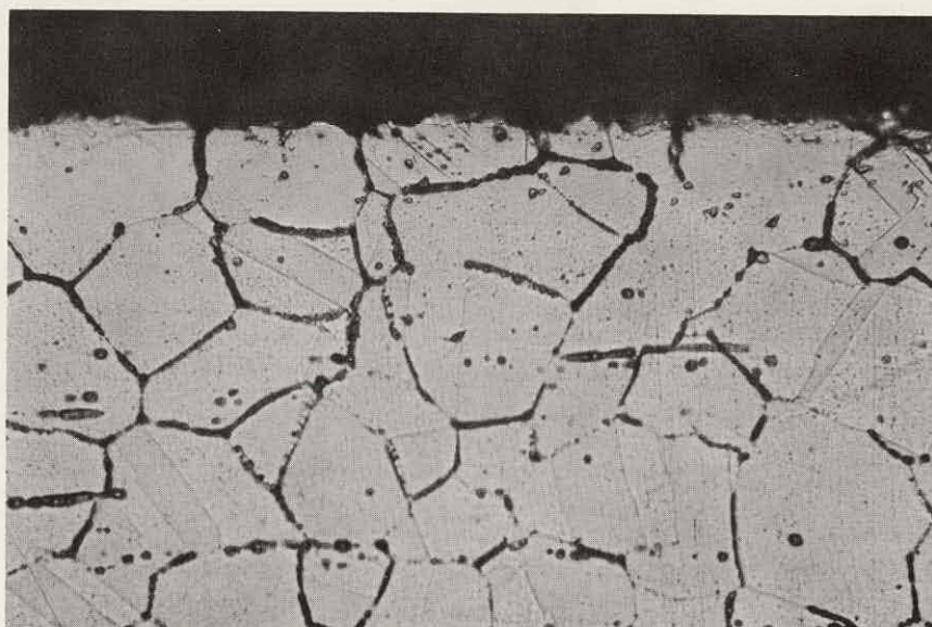
500 X Sensitized Sample Exposed for 16 Hours at 175°F and 1 gpm Oxalic Acid Etch
