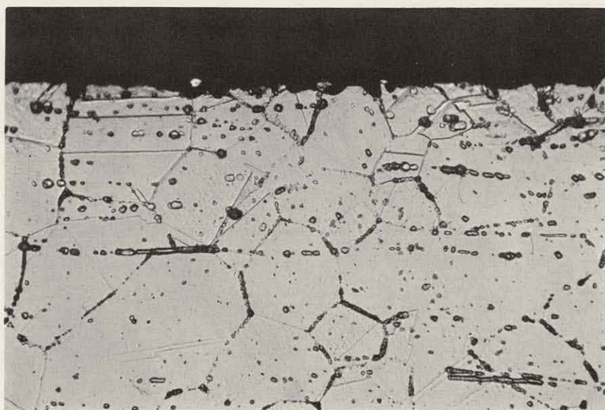
500 X Oxalic Acid Etch Sensitized Sample Exposed for 28 Days at 203°F
