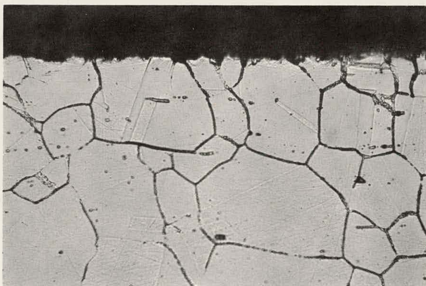
500 X Oxalic Acid Etch Sensitized Sample Exposed for 28 Days at 77°F
