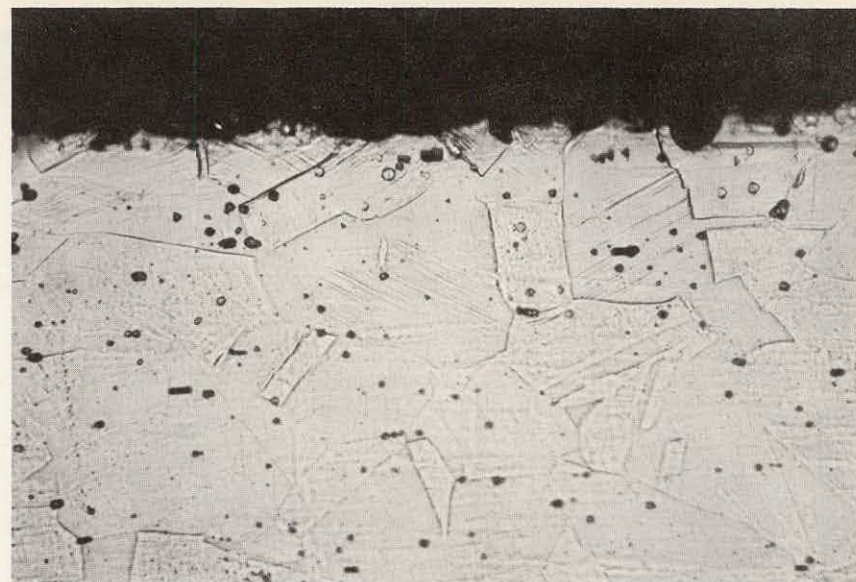
500 X Oxalic Acid Etch Annealed Specimen Outside Edge
