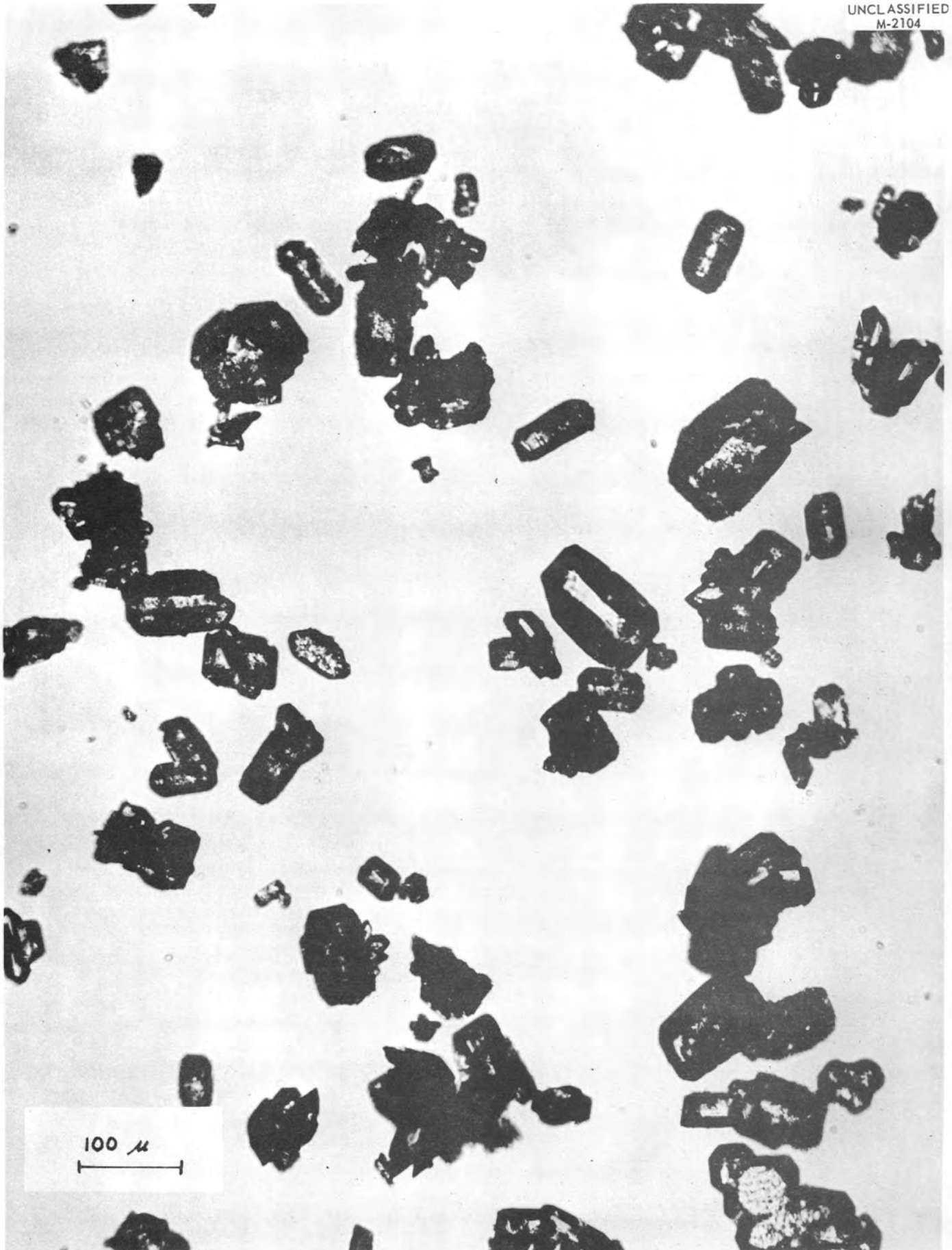
Fig. 5.3. Pseudo-Cubic Hydrate of Uranium Tetrafluoride. 200X. Reduced 10%.
