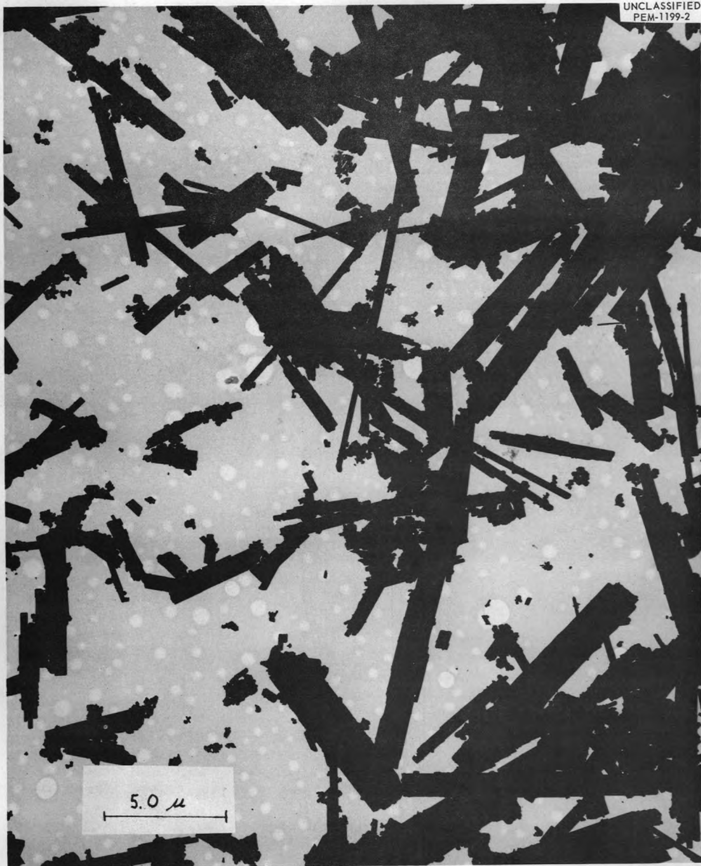
Fig. 5.1. Hydrated Uranium Tetrafluoride, \text{UF}_4 \cdot 2.5 \text{H}_2\text{O} .
