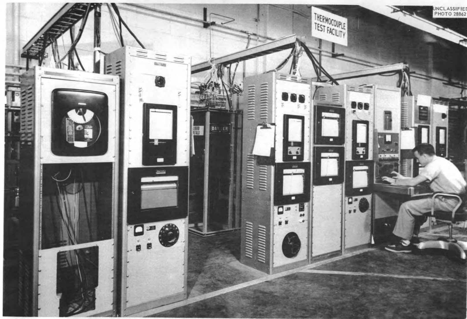
Figure 5. Facility for NaK, Na, Fluoride Salt Aging and Calibration of 0.250-in.-O.D. Sheathed and Well-Type Thermocouples. (Uncompleted cabinet will contain the controls for a eutectic salt melting point apparatus.)
