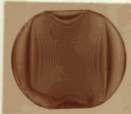
Figure 21c. Color photoplasticity fringes of the strain field
