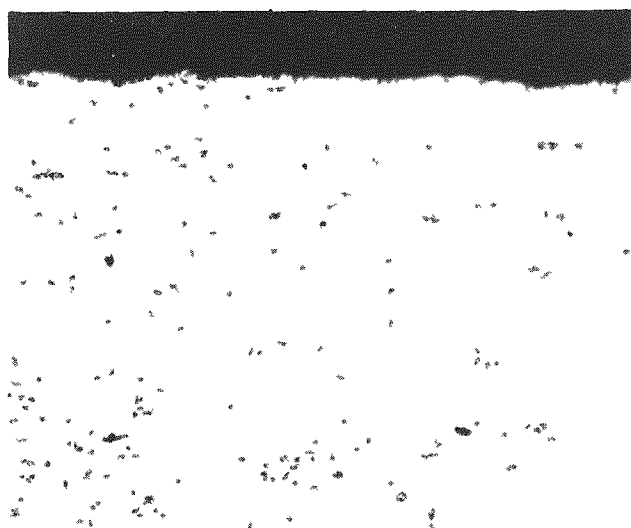
a. Outer or Gas-Metal Interface of Control Specimen F-2
