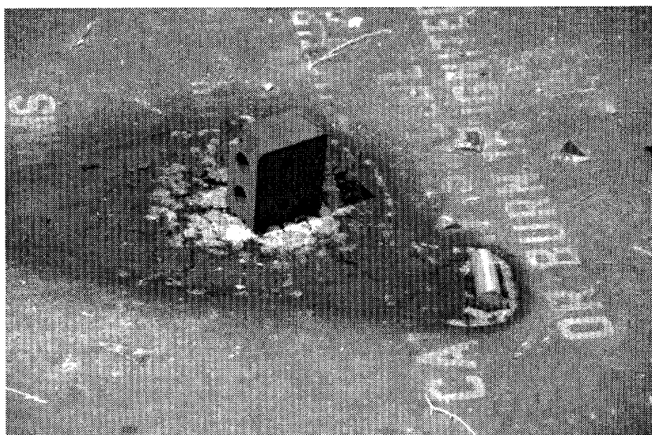
Figure 9. Ejected POCO graphite module with an ejected molybdenum slug. (Neg H-3)
