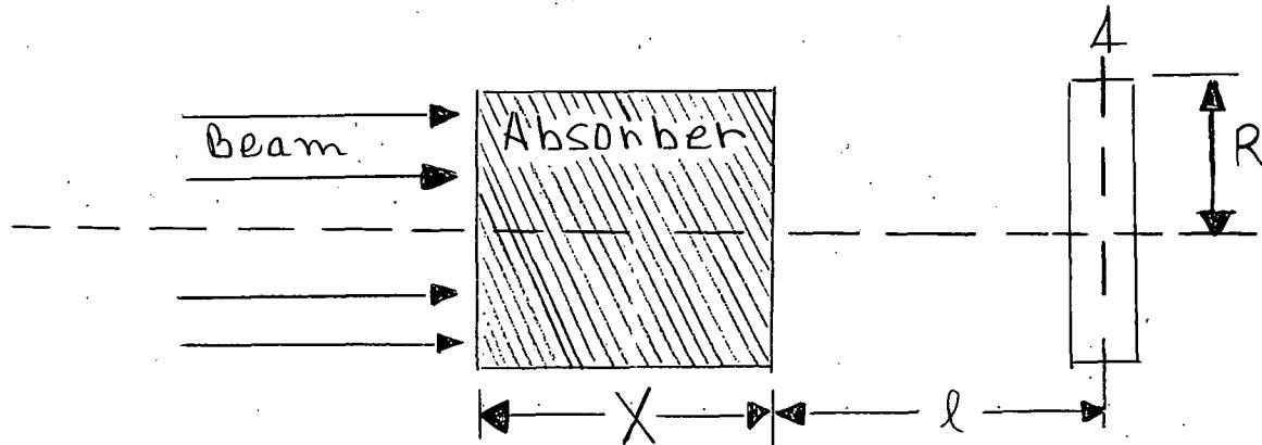
For a parallel, uniform beam of radius  $r'_0$  passing through an absorber of thickness  $x$  at a distance  $l$  from a counter of radius  $R$ , the fraction of the beam that strikes the counter is  $F(r'_0, \rho'_0)$ .  $F$  is a function of only  $\rho'_0 = r'_0/R$  and the quantity
