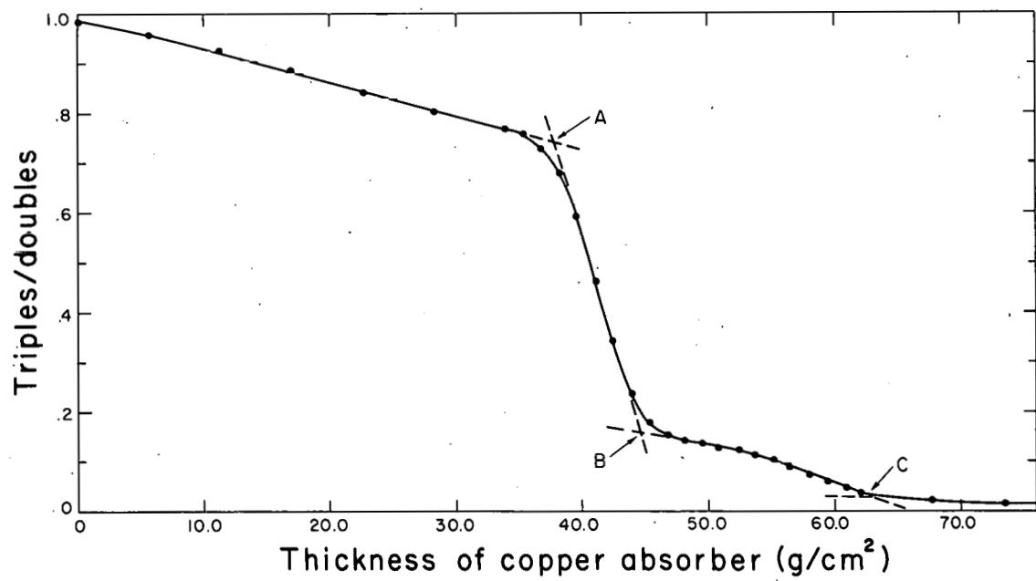
Fig. 22. Integral range curve for 102-Mev positive pion beam.
