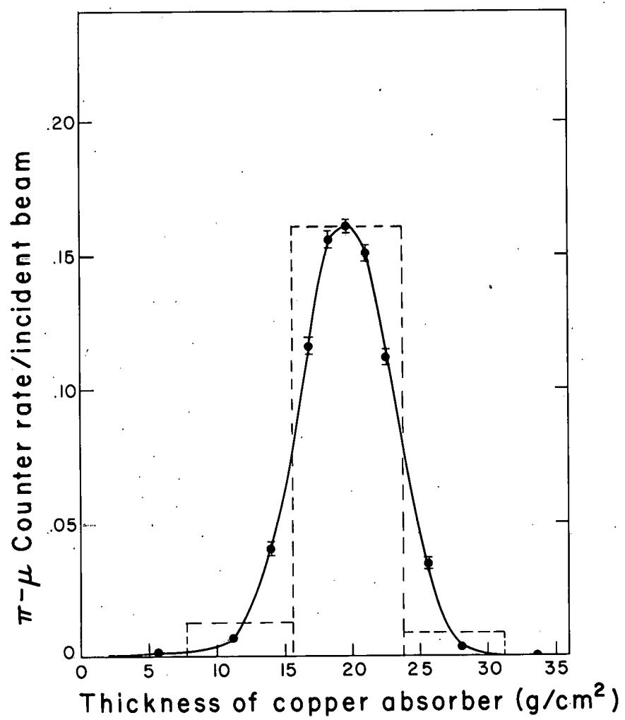
Fig. 28. Calibration curve for  $\pi-\mu$  counter telescope.
