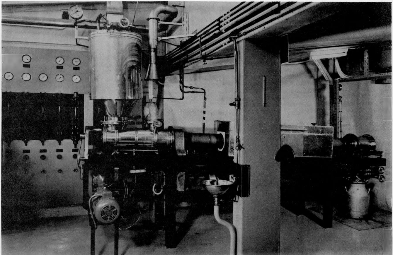
Fig. 2. Side view of the reduction furnace for UO<sub>2</sub> production.
