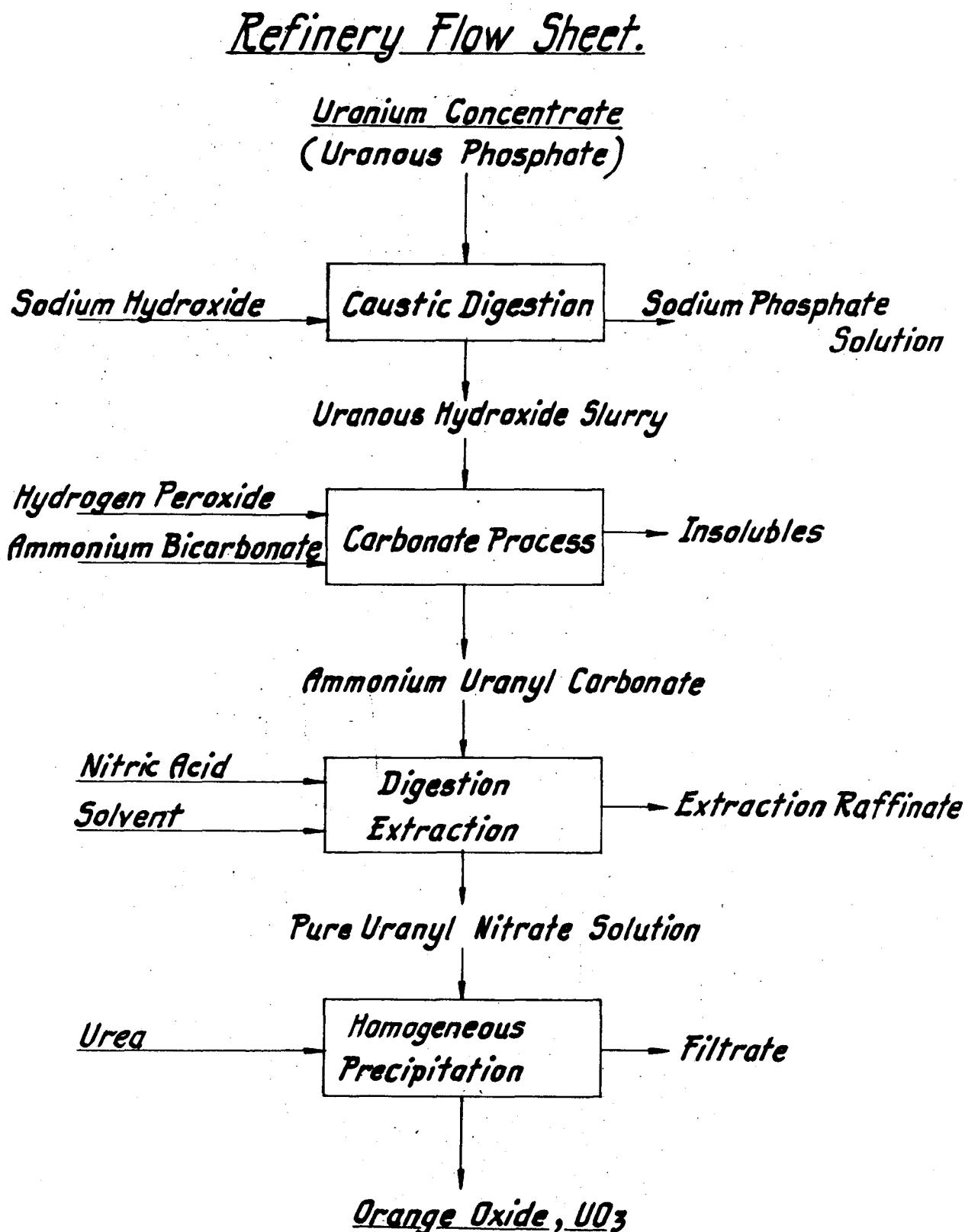
Fig. 1. Refinery Flow Sheet.
