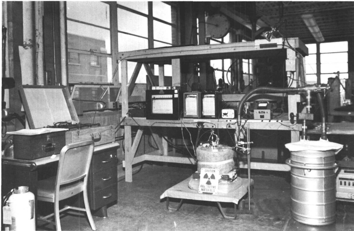
Figure 2-8. SNAP-21 Prototype Unit – Thermal Performance Test Setup
