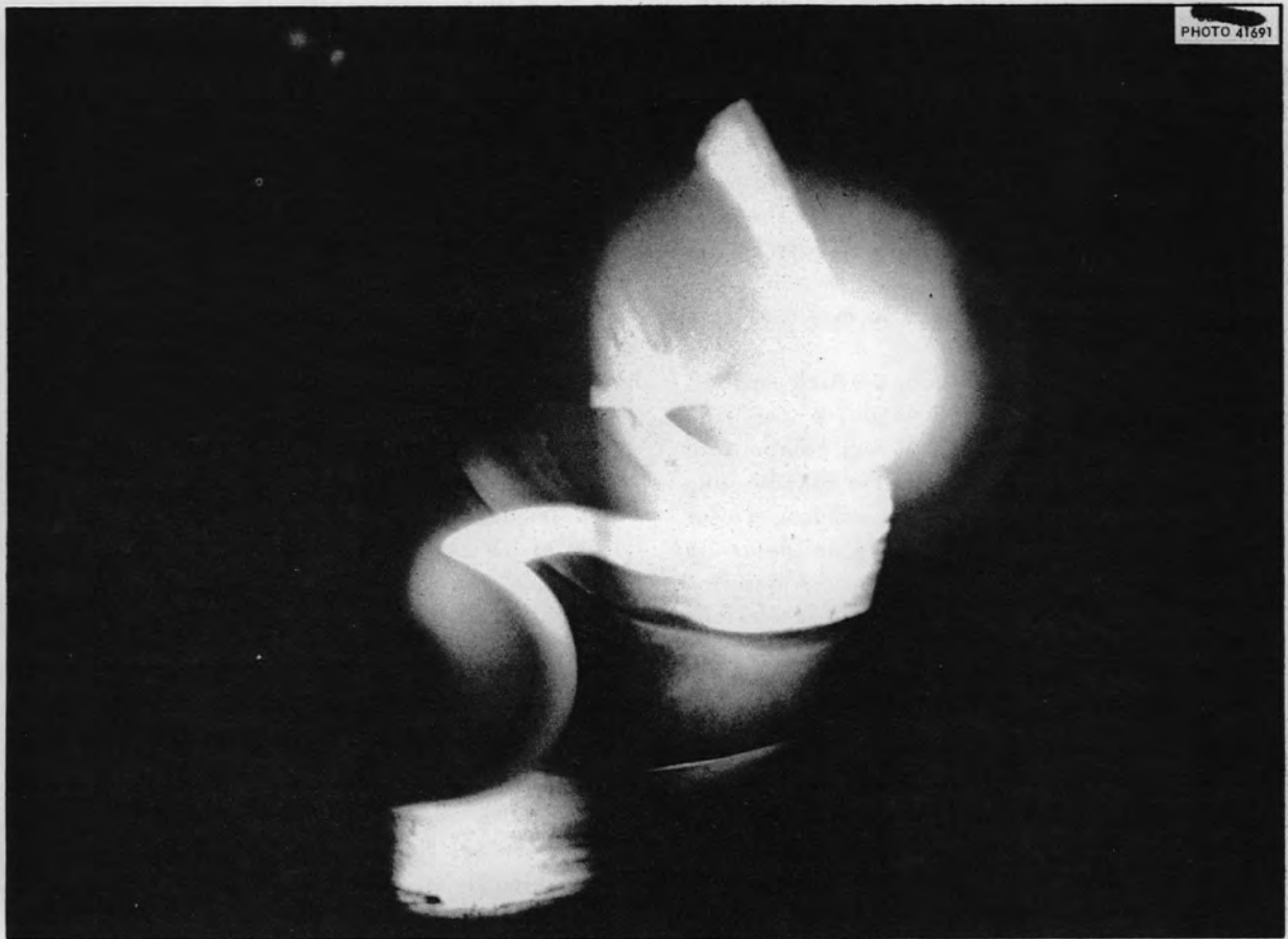
Fig. 2.2.2. Operation of the Carbon Arc in DCX. View from anode end.
