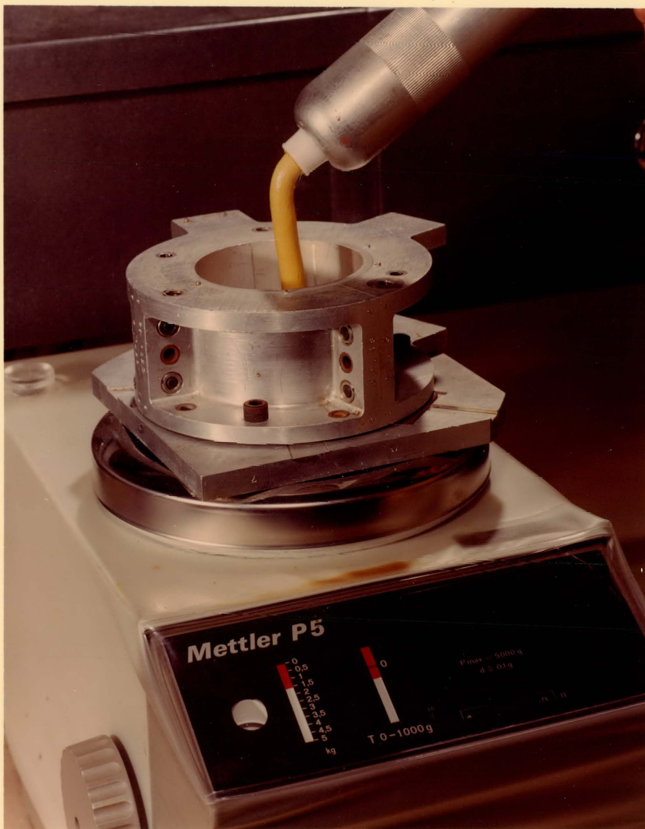
Figure 31. Extruding the Thawed Foam Premix From a Semco Tube
