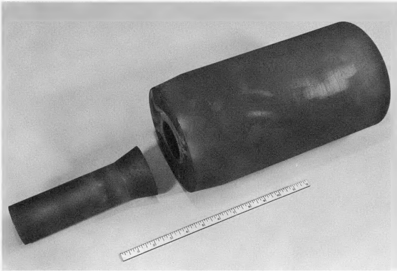
Figure 19. Graphite Crucible and Pouring Spout, Second Configuration
