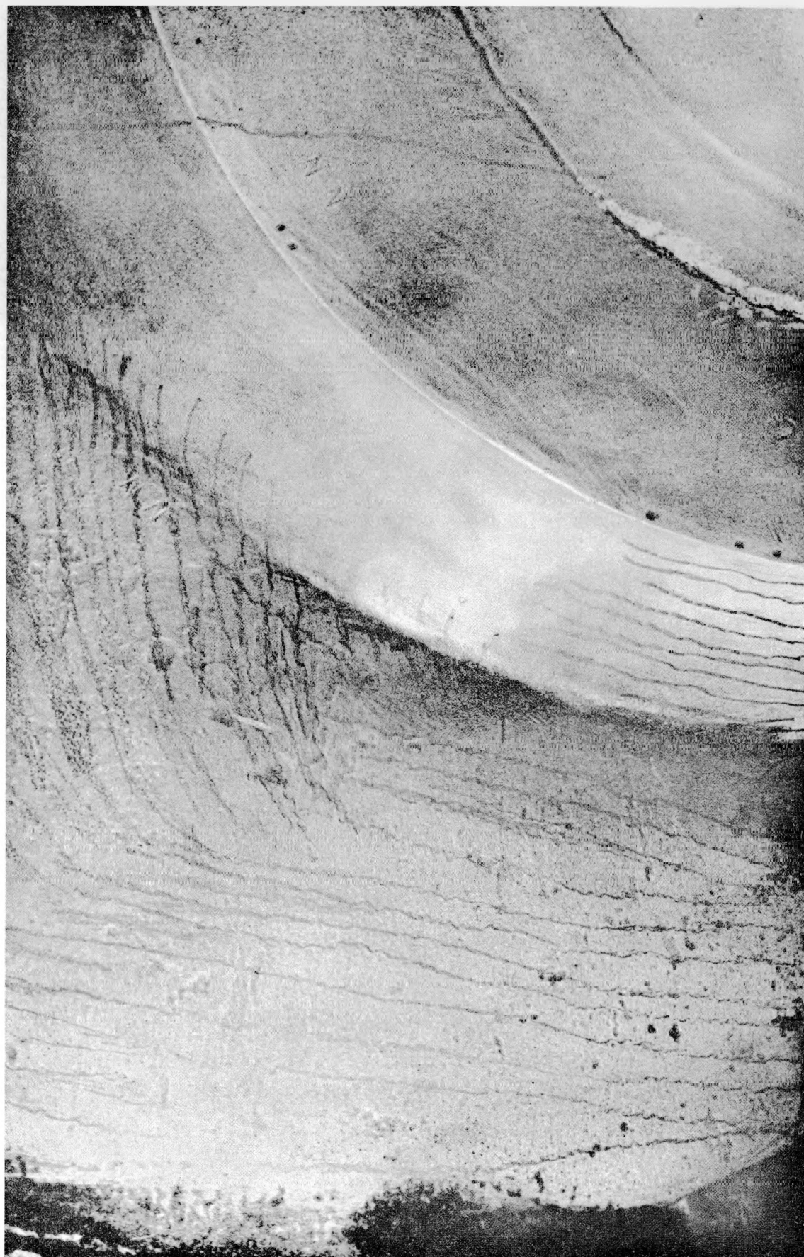
FIGURE 13. EXTERIOR SURFACE STRESSCOAT PATTERNS AT NOZZLE NO. 1
