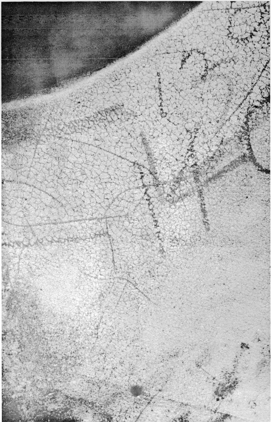
FIGURE 11. INTERIOR SURFACE STRESSCOAT PATTERNS AT RADIAL NOZZLE
