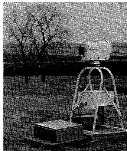
Engineers from Pacific Northwest have worked with instrument manufacturers to improve the use of multifrequency microwave radiometers to measure path-integrated water vapor and cloud liquid water.
