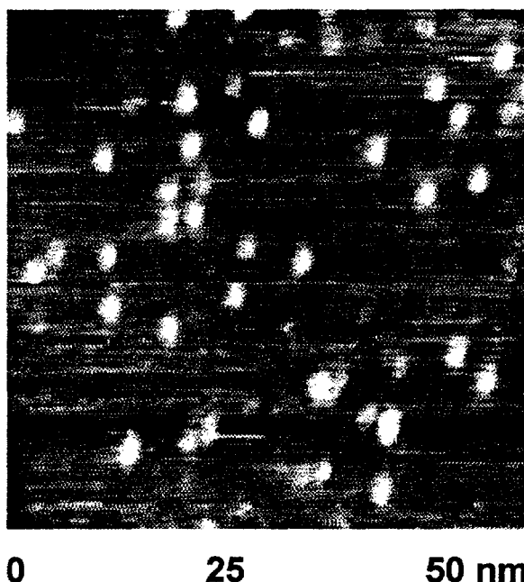
Figure 3.4 STM image of Si clusters formed on HOPG after substrate annealing to 500 °C for 5 minutes.
