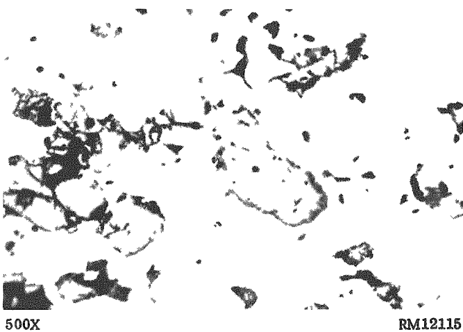
FIGURE 2. TYPICAL MICROSTRUCTURES OBTAINED IN THE STUDY OF THE COMPATIBILITY OF UN WITH NICKEL, CHROMIUM, AND IRON
