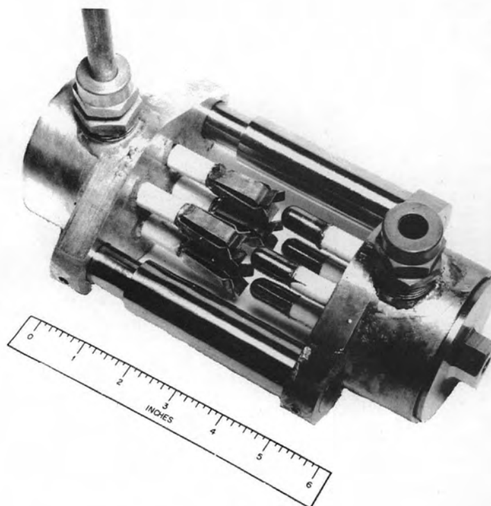
Fig. 96. Experimental Waterproof Disconnect for Mineral-Insulated Cable.
