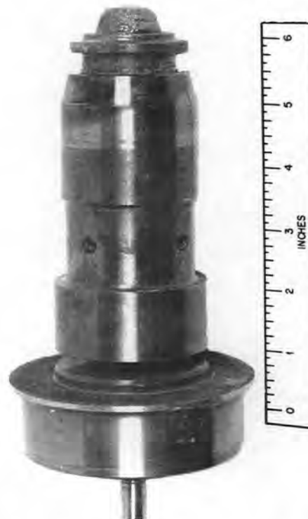
Fig. 79. Plug and Guide Assembly from High-Pressure Slurry Control Valve.
