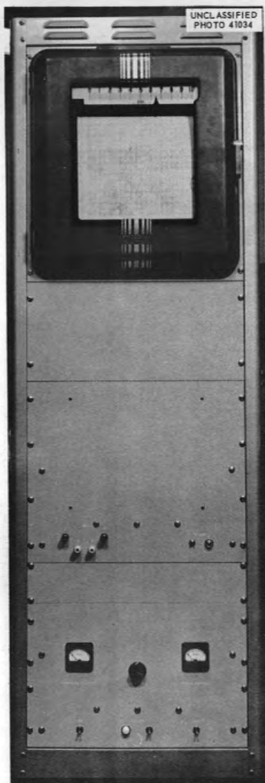
Fig. 27. Front View of Automatic Kelvin Bridge Resistance Recorder.
