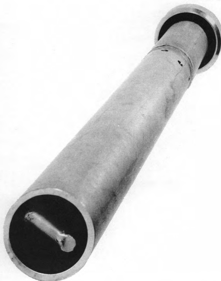
Fig. 56. Resistance-Type Fuel Level Probe Without Temperature Compensation. Lower end.
