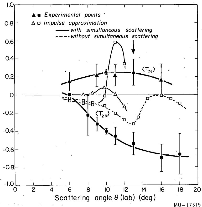
Fig. 22. (b) Polarization components for 420-Mev deuterons scattered by carbon, with impulse-approximation predictions from Hafner proton amplitudes. Total errors are indicated. The arrow designates the diffraction minimum.
