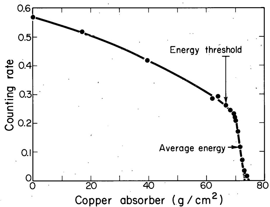
Fig. 7. (a) Range curve of beam scattered by dee target (beryllium). The energy was found equal to  $410 \pm 2.5$  Mev, and the extrapolation factor was 2.28. The energy threshold indicates the amount of absorber (except for recoil correction) used for scattering measurements.
