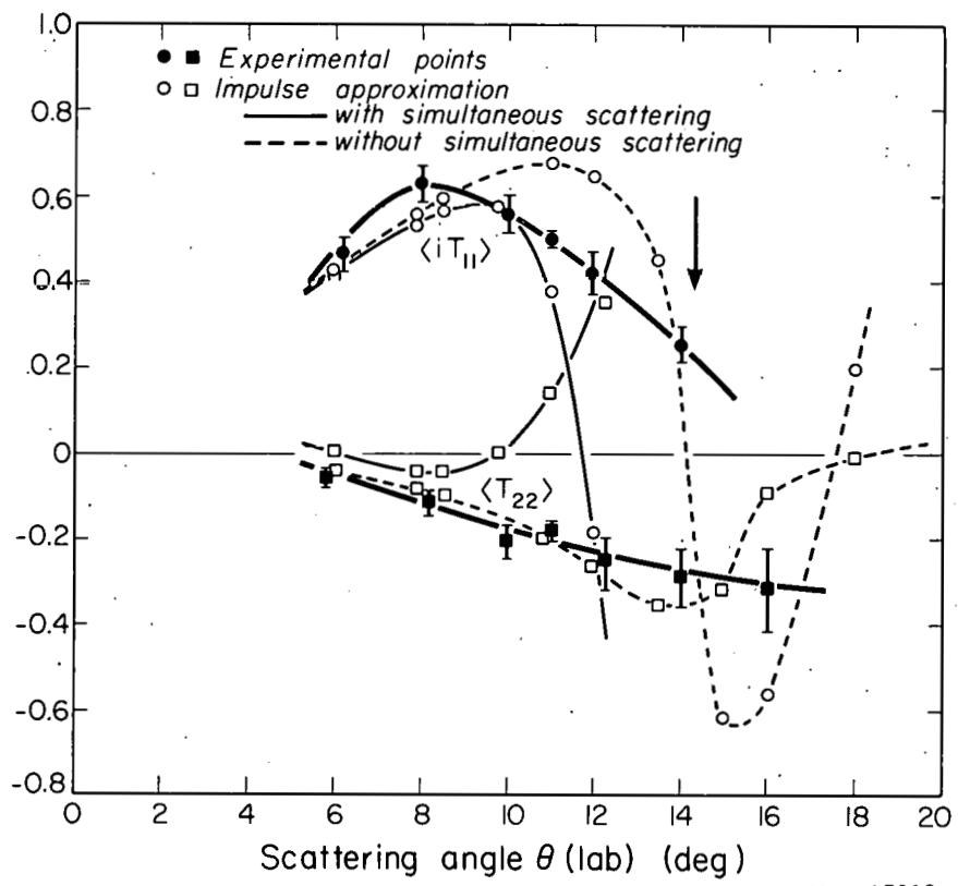
Fig. 21. (a) Polarization components for 410-Mev deuterons scattered by beryllium. Errors on experimental points include statistical and systematic effects. Impulse-approximation calculations were done with Hafner proton amplitudes. The vertical arrow indicates the position of the diffraction minimum.
