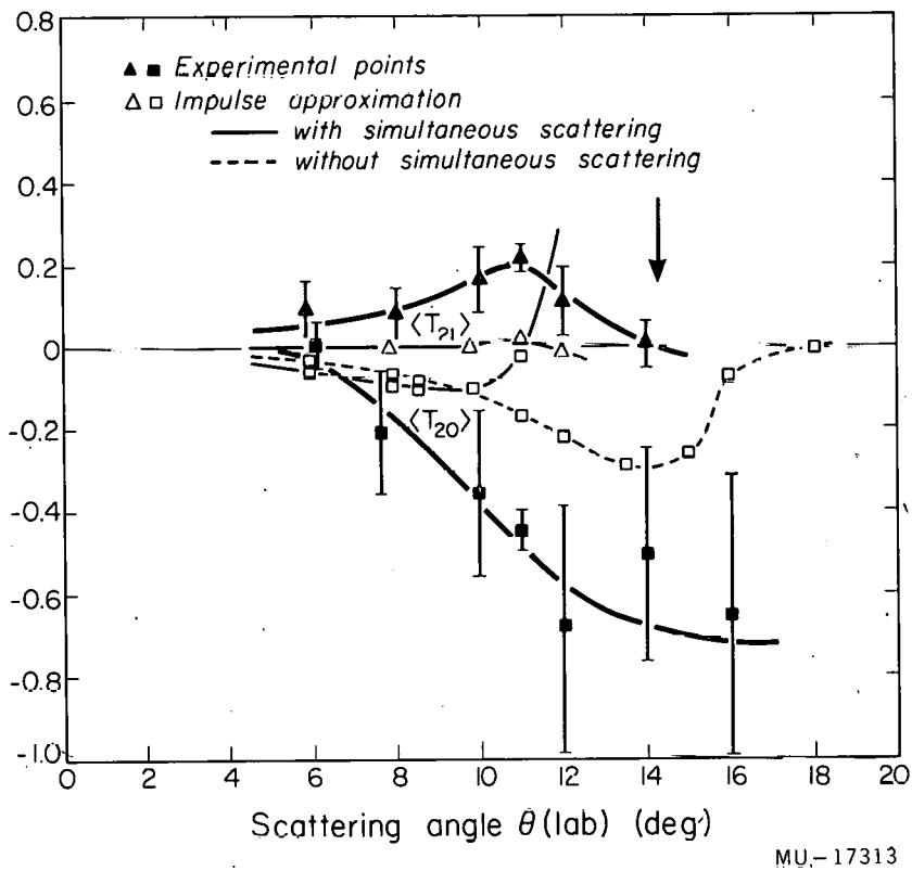
Fig. 21. (b) Polarization components for 410-Mev deuterons scattered by beryllium. Errors on experimental points include statistical and systematic effects. Impulse-approximation calculations were done with Hafner proton amplitudes. The vertical arrow indicates the position of the diffraction minimum.  $\langle T_{21} \rangle$  is zero in the usual impulse approximation.
