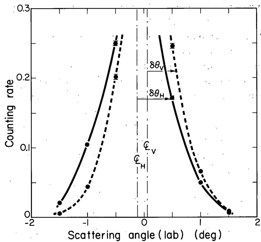
Fig. 11. Profiles of regenerated beam in horizontal plane (solid curve) and vertical plane (dotted curve);  $\delta\theta_H$  and  $\delta\theta_V$  are to be compared to an estimated resolution of 0.57 deg. Displacement of centerlines from 0 deg indicates the amount of realignment that was necessary.
