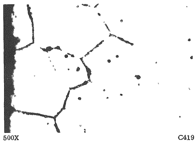
Nickel Thermocouple Tube Showing Intergranular Attack After 1000 Hr
