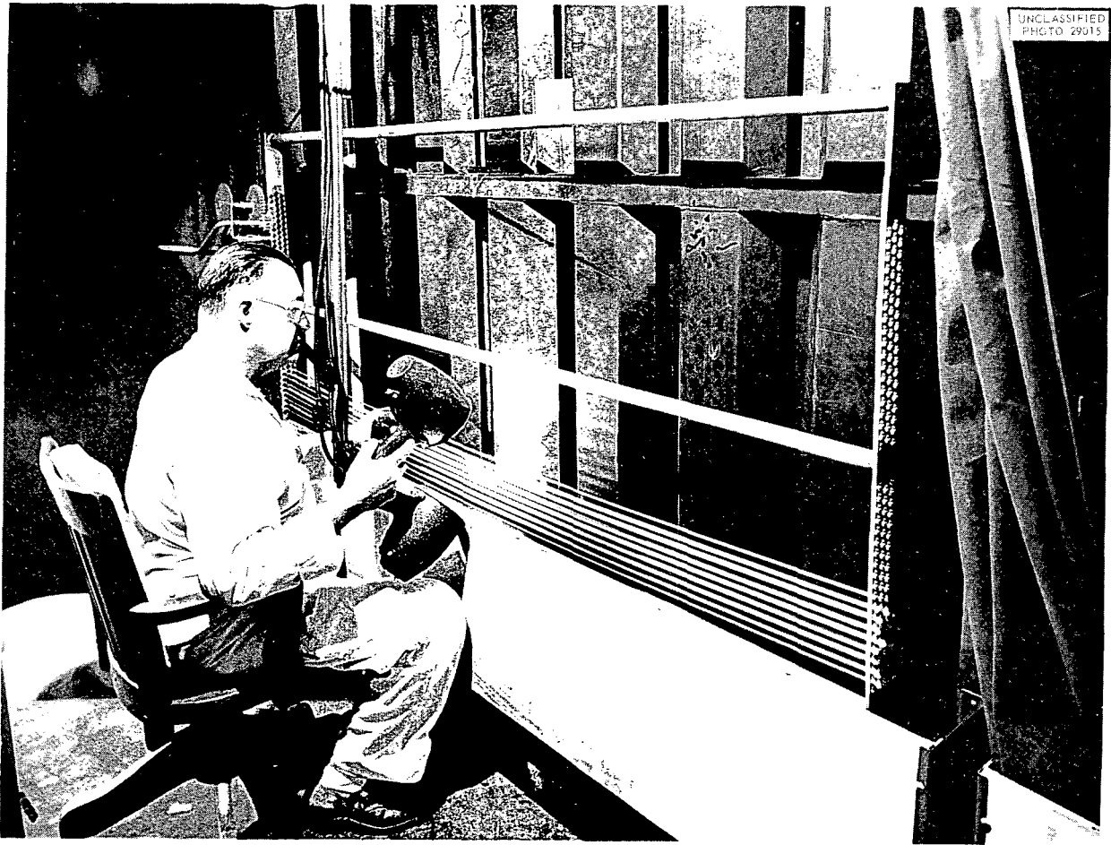
Fig. 26. Rack of Small-Diameter Tubes Being Inspected with Use of Black Lights.
