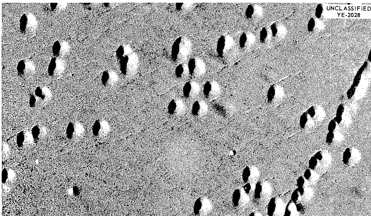
Fig. 139. Inconel Cathodically Etched in Vacuum. Formvar replica shadowed with gold-Manganin alloy. While not obvious here, lower magnification shows the characteristic alignment of the precipitate. 22,500X.
