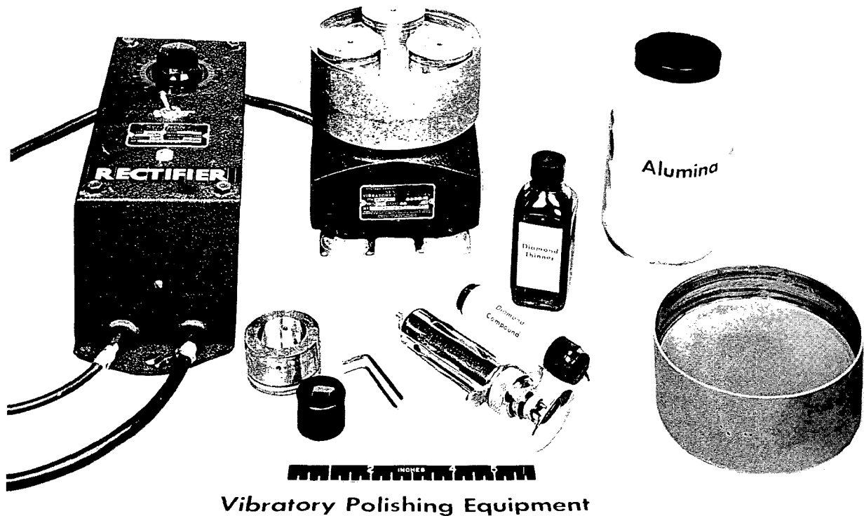
Fig. 129. Small Vibratory Polisher (5-in.-dia Bowl) Employed in Initial Investigation.
