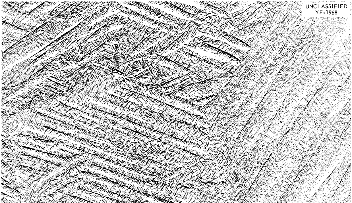
Fig. 46. Carbon Replica, Preshadowed with Gold-Manganin, of Tantalum Specimen Oxidized for 24 hr at 400°C. 12,000X.
