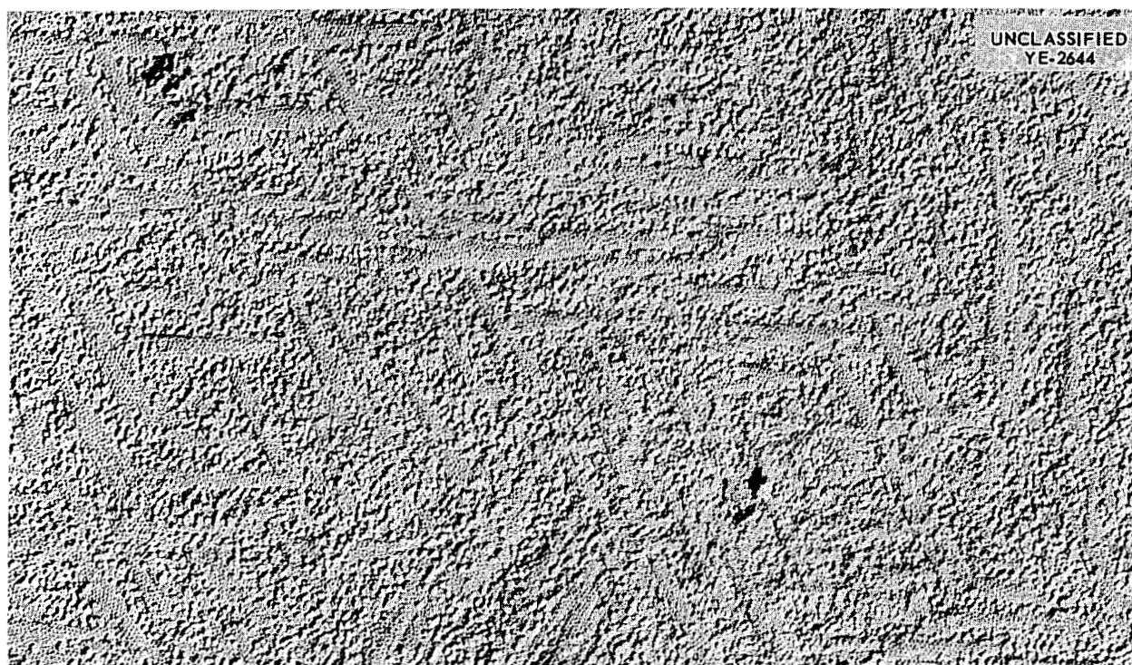
Fig. 55a. Carbon Replica, Preshadowed with Gold-Manganin, of Tantalum Specimen Sulfurized for 24 hr at 425°C. 12,000X.
