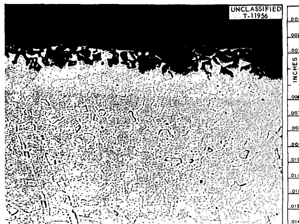
Fig. 20. Maximum Hot-Leg Attack Observed in Niobium Loop 1072, Which Operated 1664 hr with Fuel No. 107 at 1500°F. 250X. Reduced 32%. (Secret with caption)
