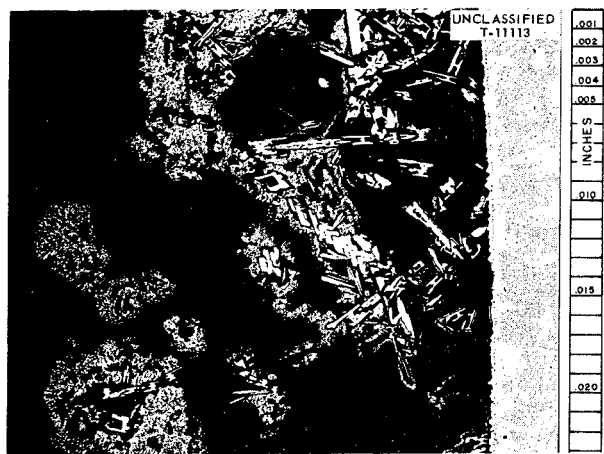
Fig. 12. Appearance of Mass Transfer Deposits in Inconel Loop 7426-17, Which Circulated NaK at 1500°F. Cold trap was maintained at 800°F. 150X. Reduced 31.5%.
