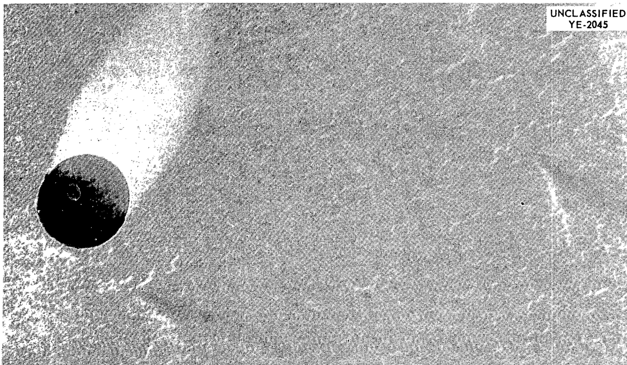
Fig. 138. Inconel Etched with Glyceria Regia. Sphere placed on surface to determine shadowing direction. Formvar replica shadowed with gold-Manganin alloy. Same replica as in Fig. 137. Shadows cast by "sharks teeth" can be correlated with shadow of ball. 90,000X.
