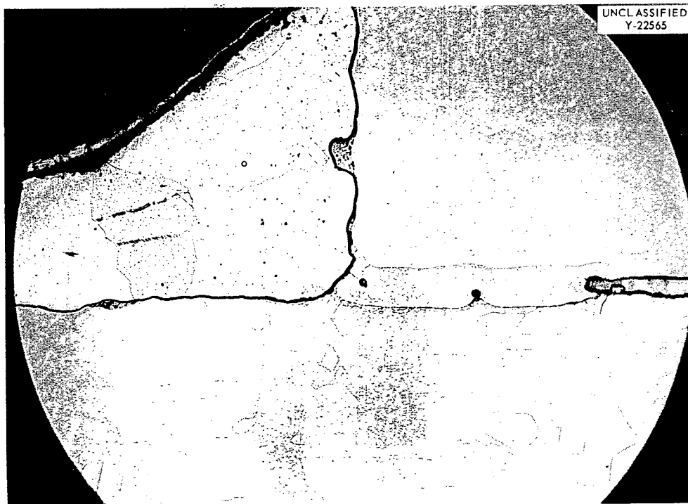
Fig. 131. Photomicrograph of Ni-V-Ag Junction with Ag Solder Weld. Etchant: 50% KCN- (\text{NH}_4)_2\text{S}_2\text{O}_8 and glycerine. 50X. Reduced 19%.
