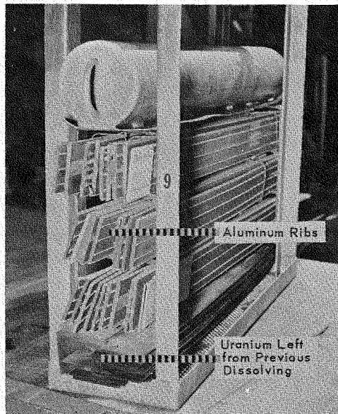
FIGURE 9 - CHARGE OF FLAT PLATES AFTER PARTIAL DEJACKETING
