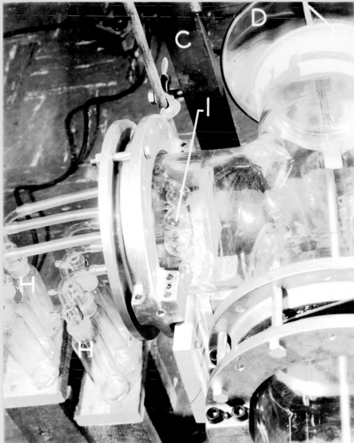
a. Impinger Assembly Attached to 6-Inch Diameter Coalescence Tube
