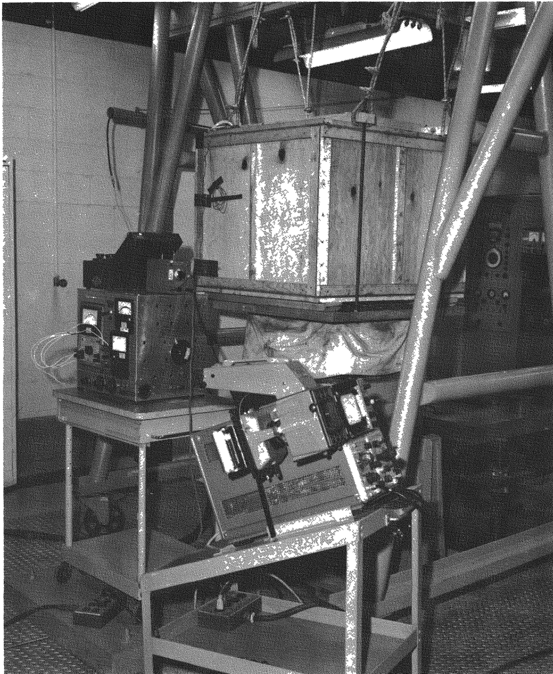
Fig. III-14. Equipment Setup for Vertical Vibration Testing
