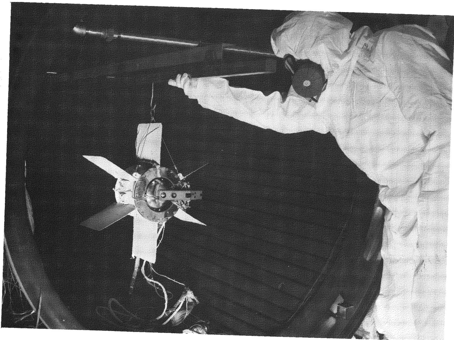
Fig. V-18. SNAP 11 Generator in Lunar Simulation Chamber
