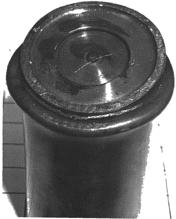
FIG. III-20. FAILURE IN THE WELD AREA
