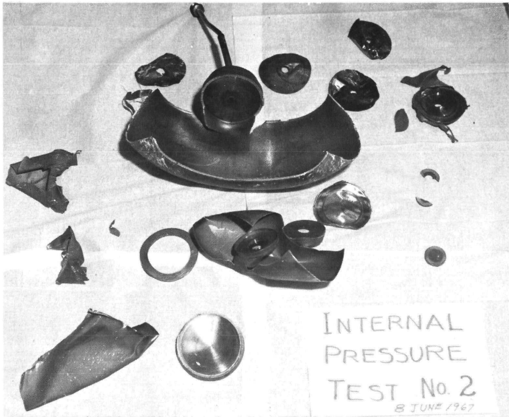
FIG. III-13. POST-TEST RUPTURE AT 5800 PSIG
