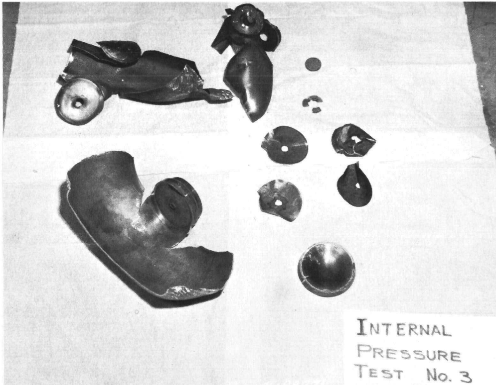
FIG. III-14. POST-TEST RUPTURE AT 6400 PSIG
