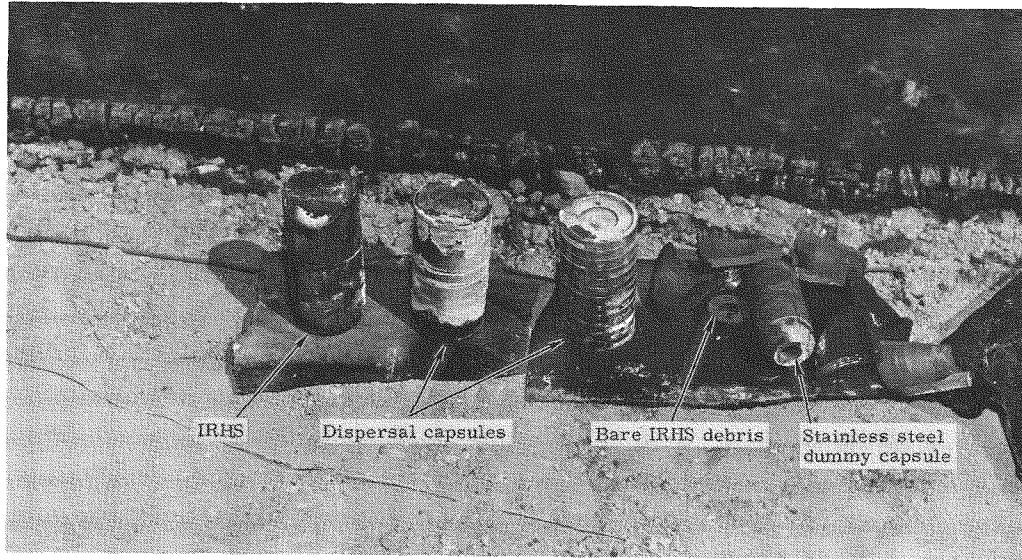
FIG. IV-49. IRHS AND DISPERSAL HEAT SOURCES AFTER RESIDUAL FIRE TEST
