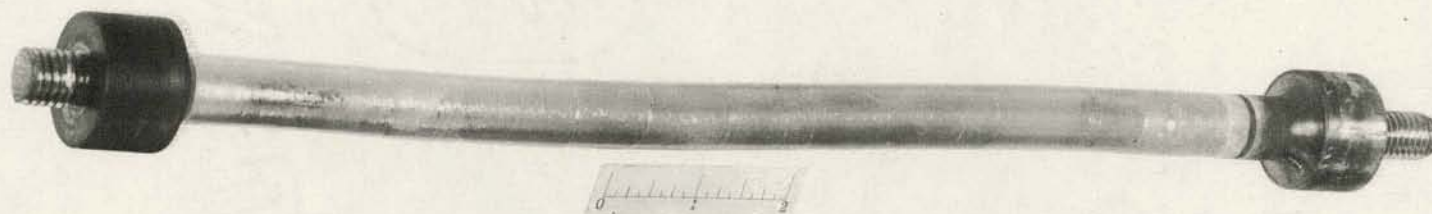
Fig. III - Yttrium metal bar after 200 hour electrolysis at 2200°F. (U37026A)
