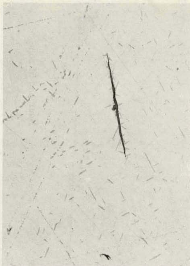
Fig. 1 - Microstructure of typical yttrium metal from Ames Process. Etched with H_3PO_4 in glycerin and ethylene glycol. (X250)
