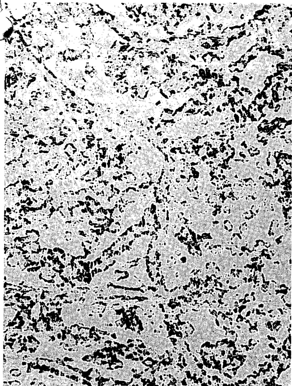
Fig. 25 x150 Alloy 19 40 d 700°C w.q. polish attack
