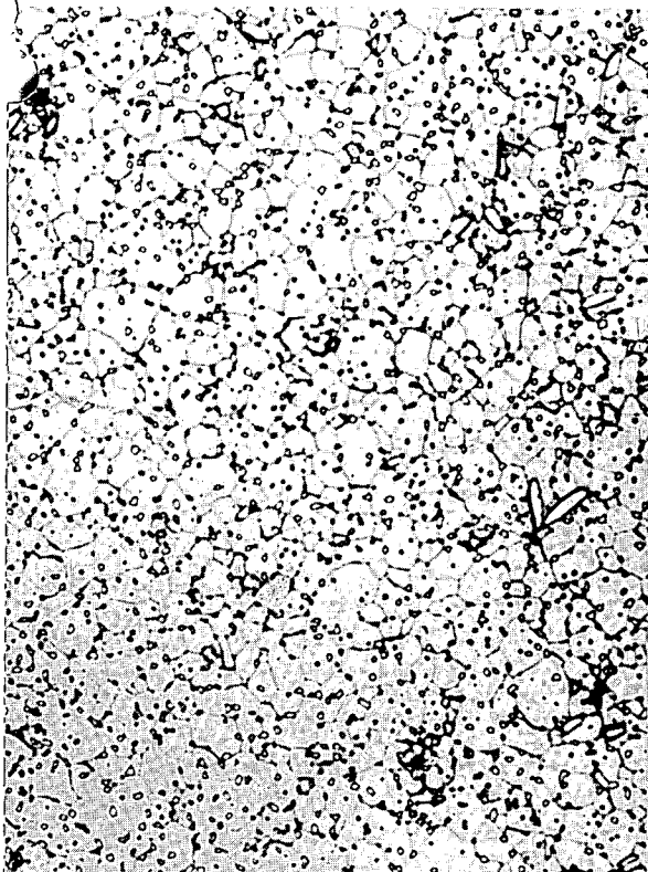
Fig. 14 x500 U-20 a/o Nb-18 d 600°C w.q. oxalic etch.
