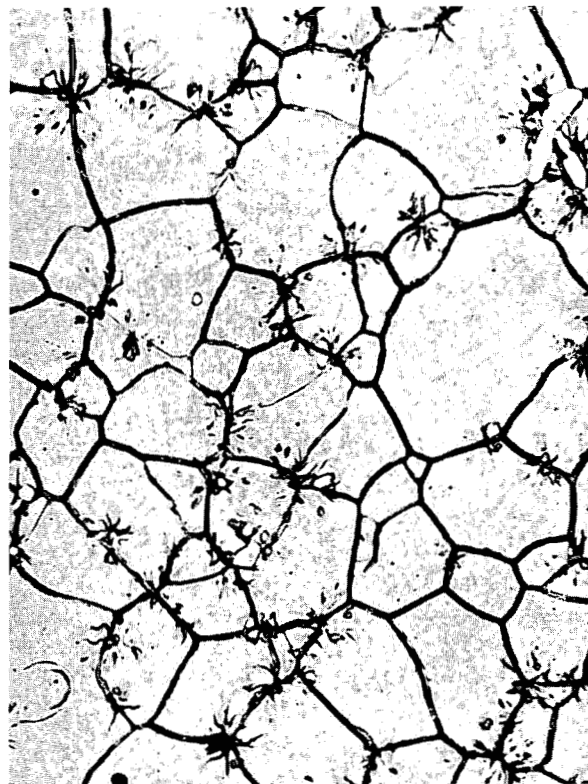
Fig. 11. x500 U-15 a/o Nb + 8d at 660°C w.q. oxalic acid etch.
