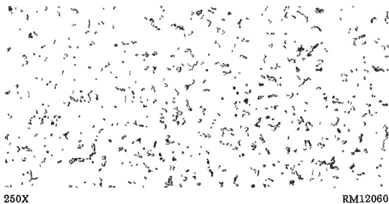
FIGURE 8. IRON-49 w/o CHROMIUM-5.2 w/o YTTRIUM ALLOY HELD 10 DAYS AT 900 C AND WATER QUENCHED
