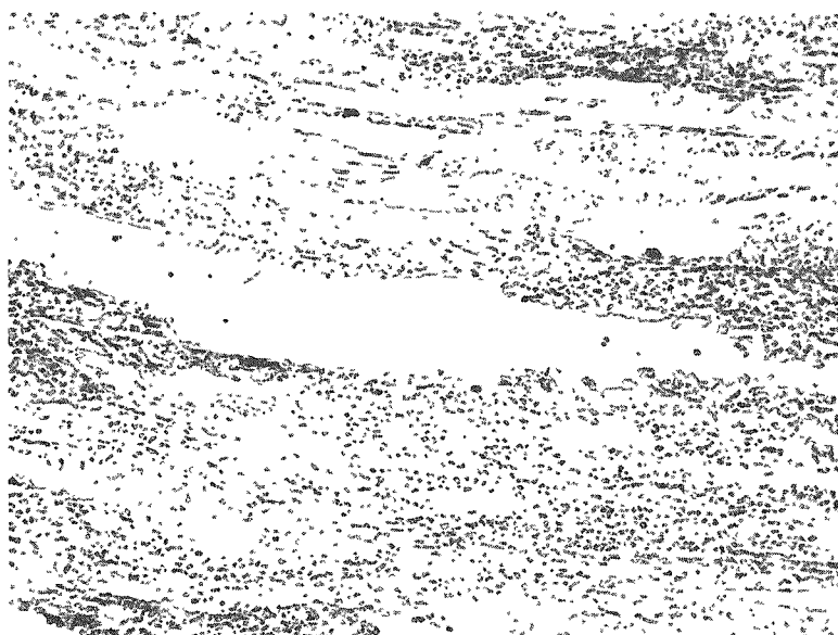
FIGURE 11. IRON-40 w/o CHROMIUM ALLOY HELD 3 MONTHS AT 600 C AND WATER QUENCHED
