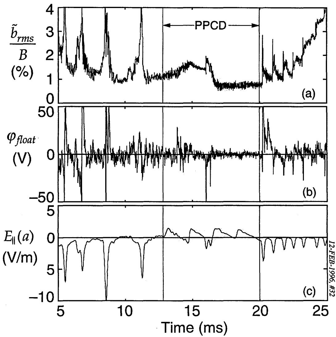
Fig. 2, *Reduction of Magnetic Fluctuations and Transport by Inductive Poloidal Current Drive*, J.S. Sarff et al.,
