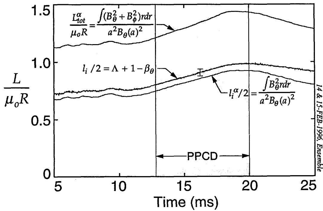
Fig. 4, Reduction of Magnetic Fluctuations and Transport by Inductive Poloidal Current Drive, J.S. Sarff et al.,
