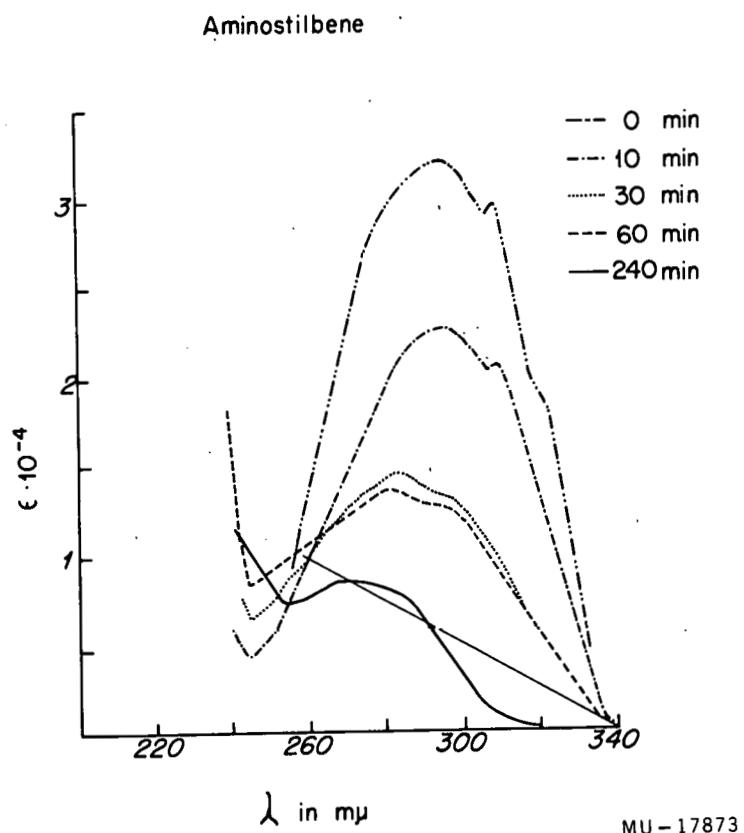
Fig. 28. Irradiation of trans p-Aminostilbene in 50% ethanol
