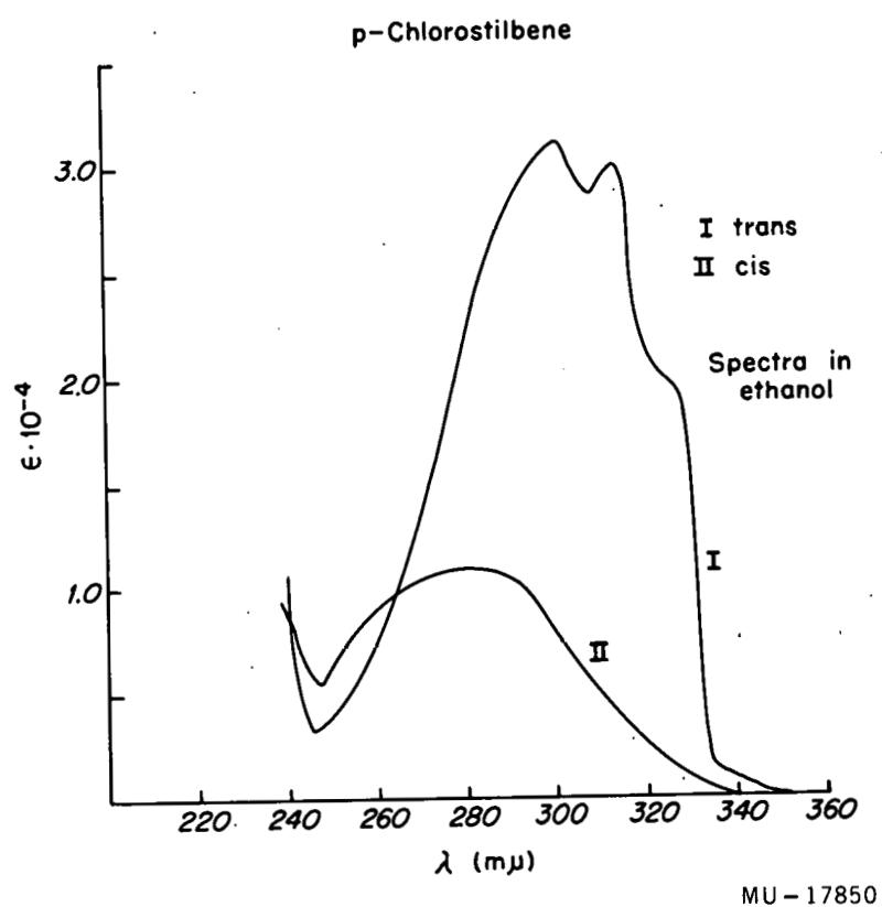
Fig. 5. Ultraviolet spectrum of p-chlorostilbenes in ethanol.
