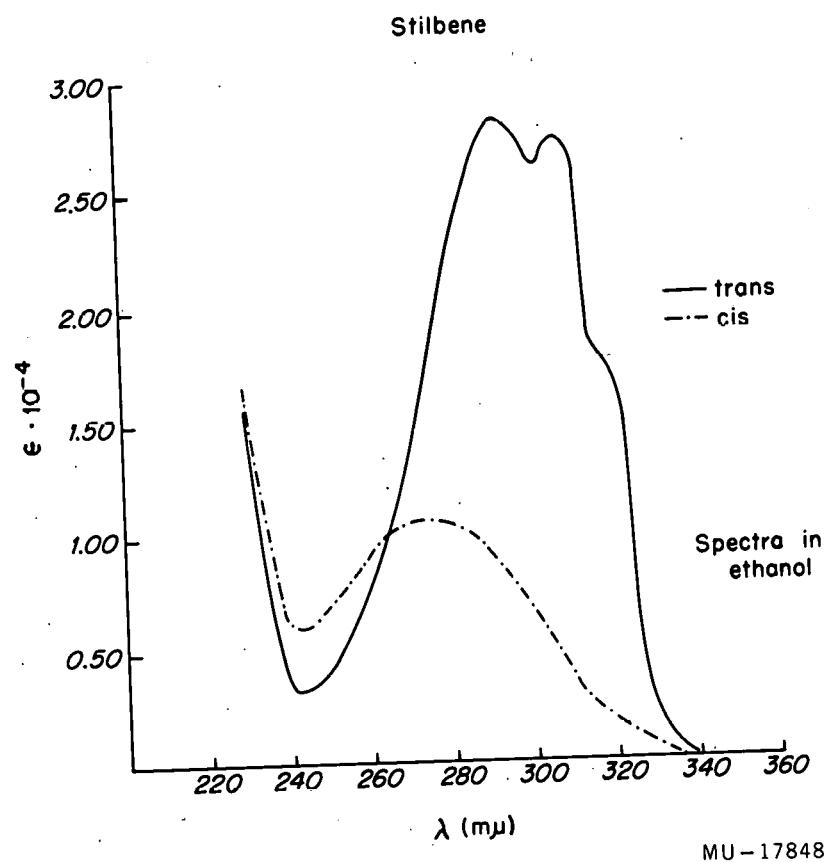
Fig. 3. Ultraviolet spectrum of cis and trans stilbene in ethanol.
