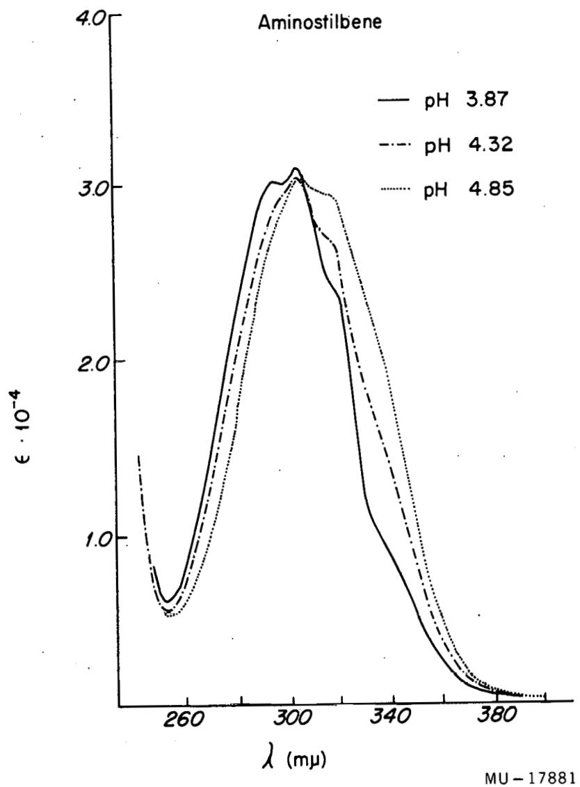
Fig. 36. Spectra of trans p-Aminostilbene at various pH in 30% methanol.
