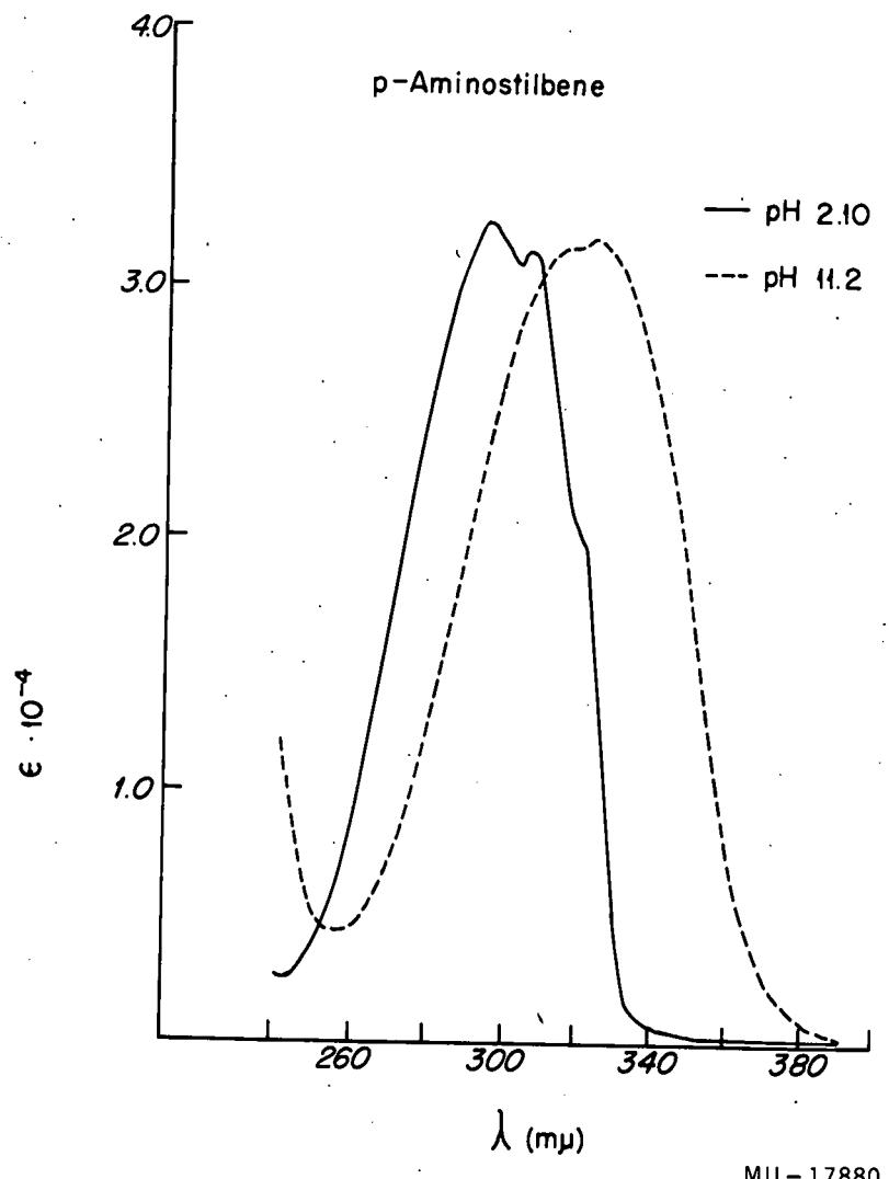
Fig. 35. Spectrum of trans p-Aminostilbene and its cation in 30% methanol.
