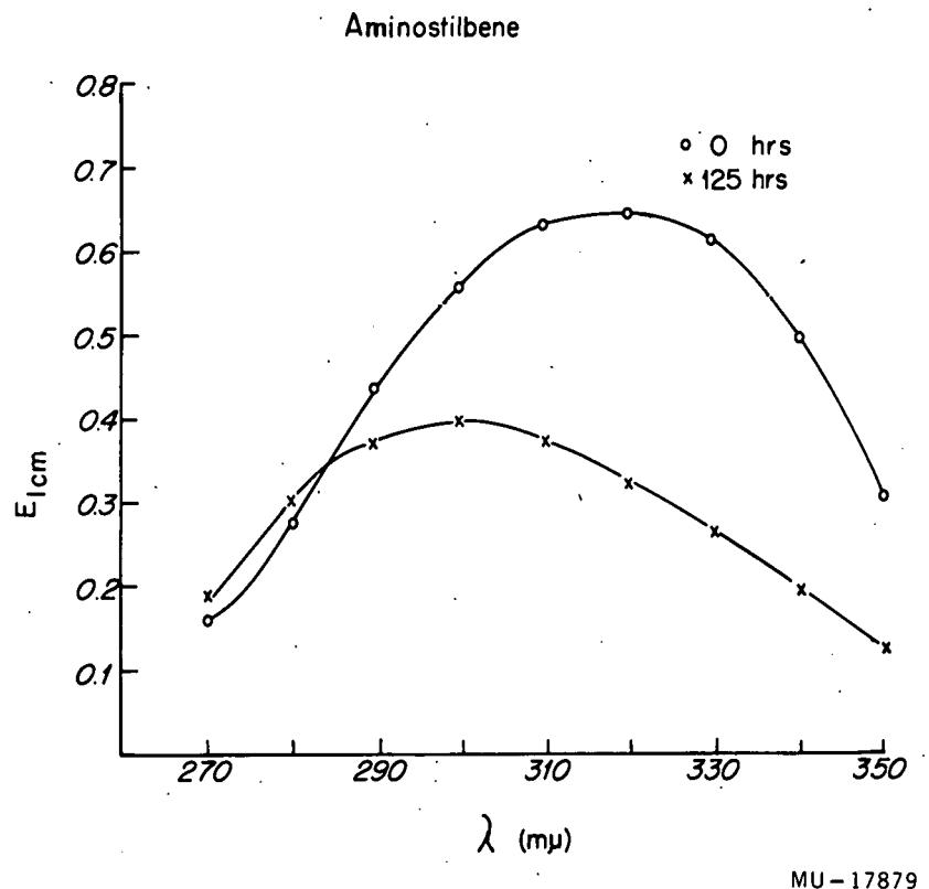
Fig. 34. Stability of trans p-Aminostilbene in 30% methanol-buffer of pH 11.2 at 25°C.
