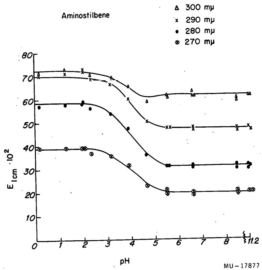
Fig. 32. trans p-Aminostilbene Change of spectrum as a function of pH.
