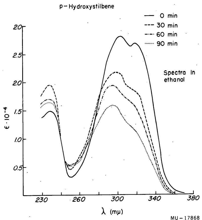
Fig. 23. Irradiation of trans p-Hydroxystilbene in ethanol
