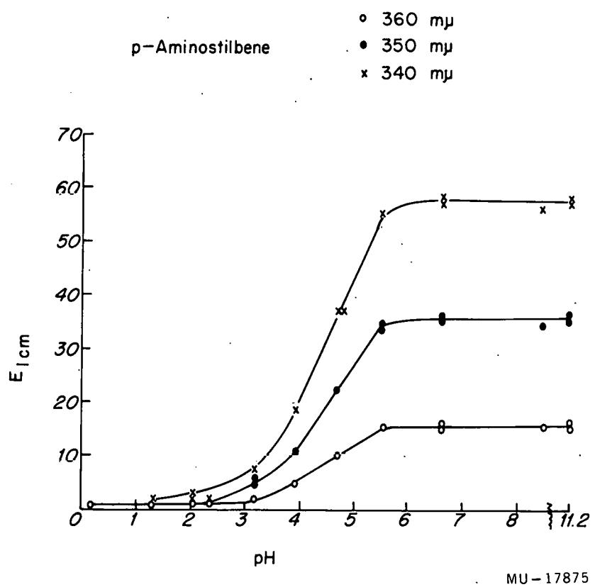
Fig. 30. *trans* *p*-Aminostilbene Change of spectrum as a function of pH.
