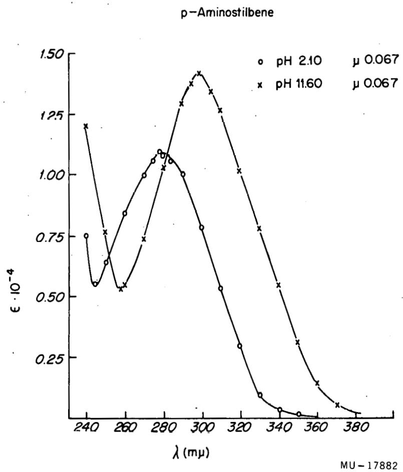
Fig. 37. Spectrum of cis p-Aminostilbene and its cation in 30% methanol.
