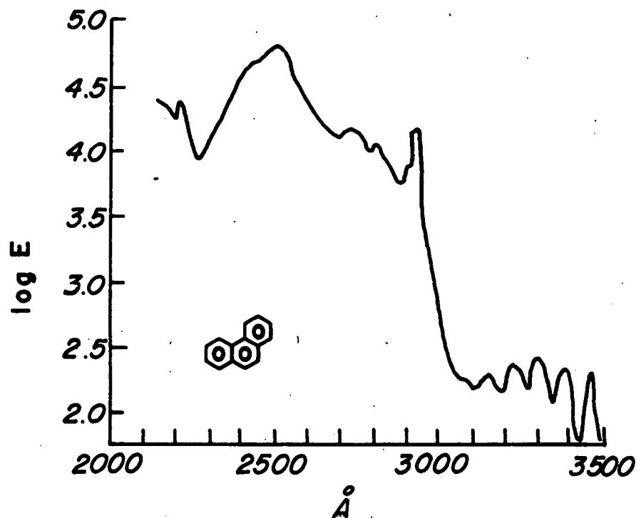
Fig. 21. Spectrum of Phenanthrene in cyclohexane.
