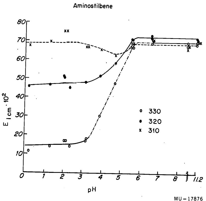
Fig. 31. trans p-Aminostilbene Change of spectrum as a function of pH.
