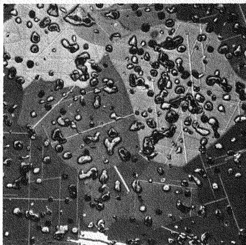
Fig. 3.1 — UC from Batch No. 1 — 500 × — nitric acid-acetic acid-water etch. The matrix phase is UC. The acicular phase is UC_2 and the globular phase may be UCO_2 . The UC and UC_2 may contain some oxygen in solid solution.
