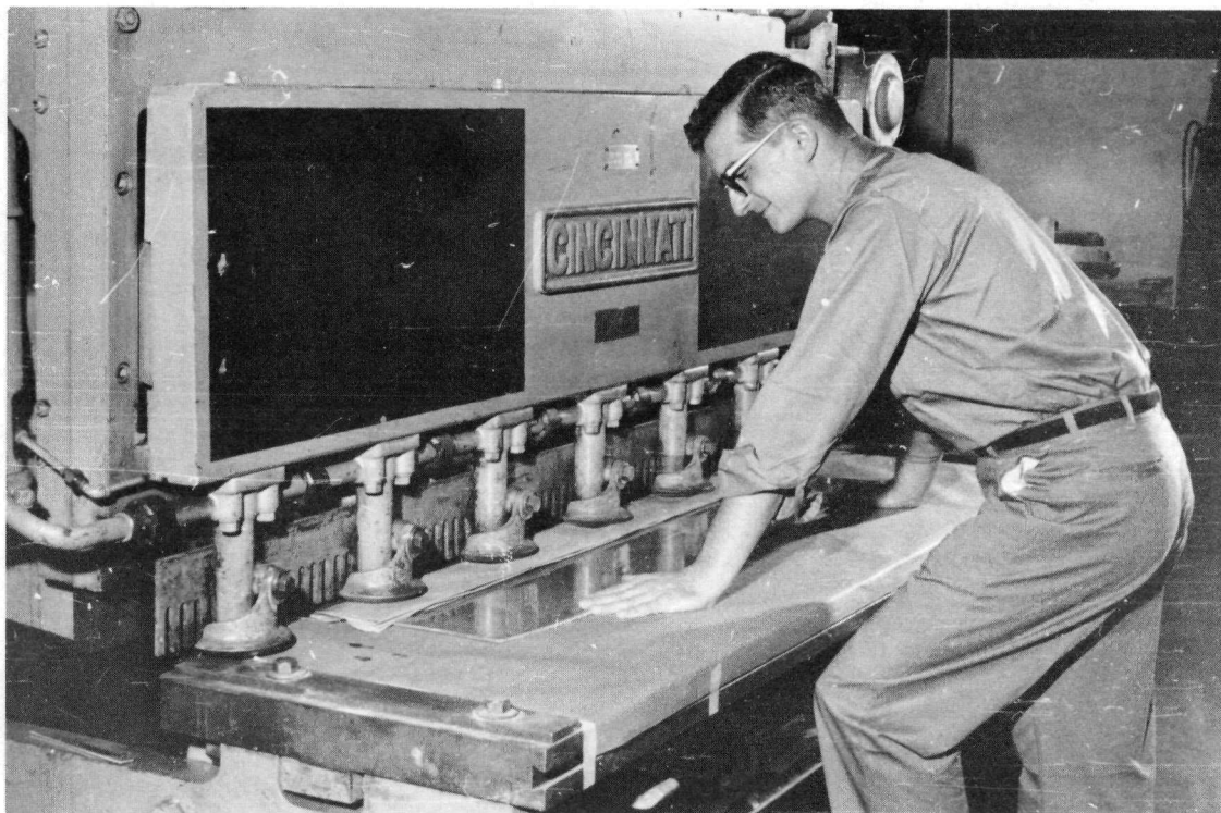
FIGURE 18. Shearing of Rolled Plate into Strips for Core Blank Punching
